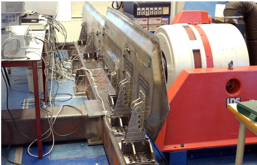
**Fig. 11** Test set-up for acoustic fatigue of a Fibre Metal Laminate (FML) weapon bay door
