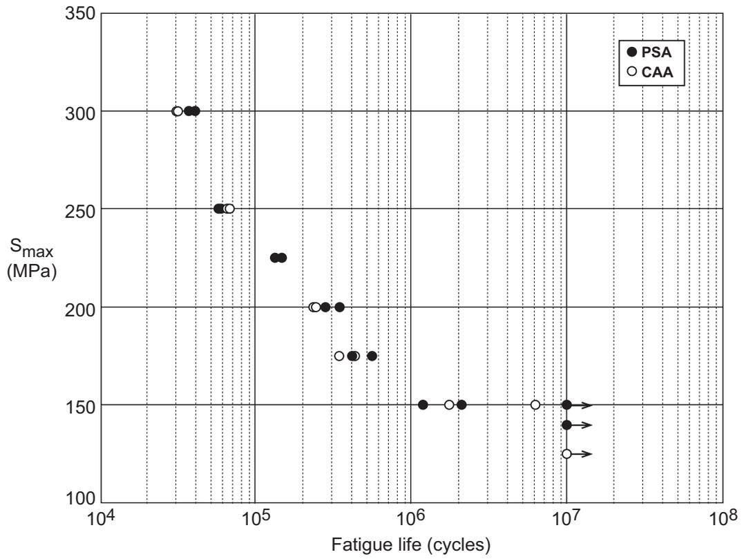
**Fig. 6 Comparison of PSA anodised and chromic acid anodised 7075-T6 clad fatigue specimens,  $K_t = 1.06$ ,  $R = 0.1$ : (see subsection 1.5.3)**
