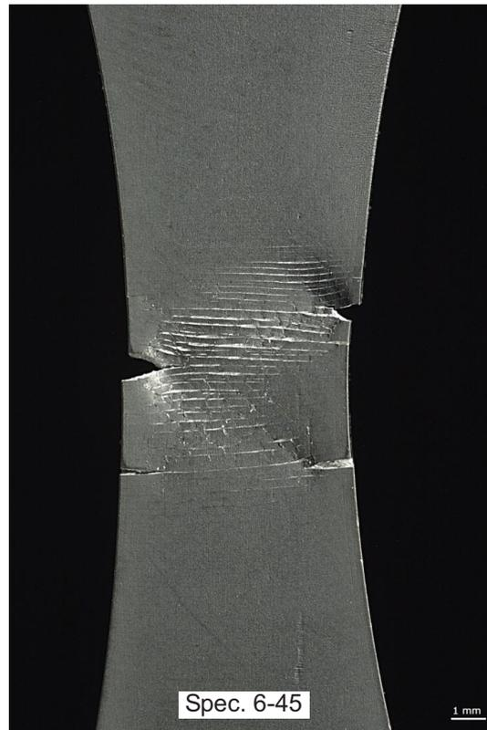
Fig. 7b Example of multiple fatigue crack initiation in a DLC coated specimen [Ref. 8]
