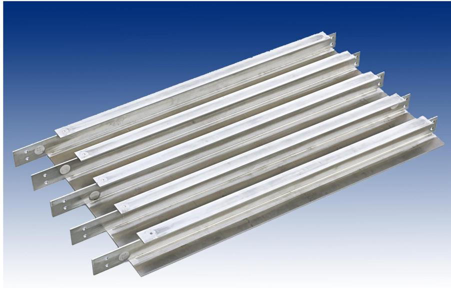
a) Stiffened panel manufactured by FSW
