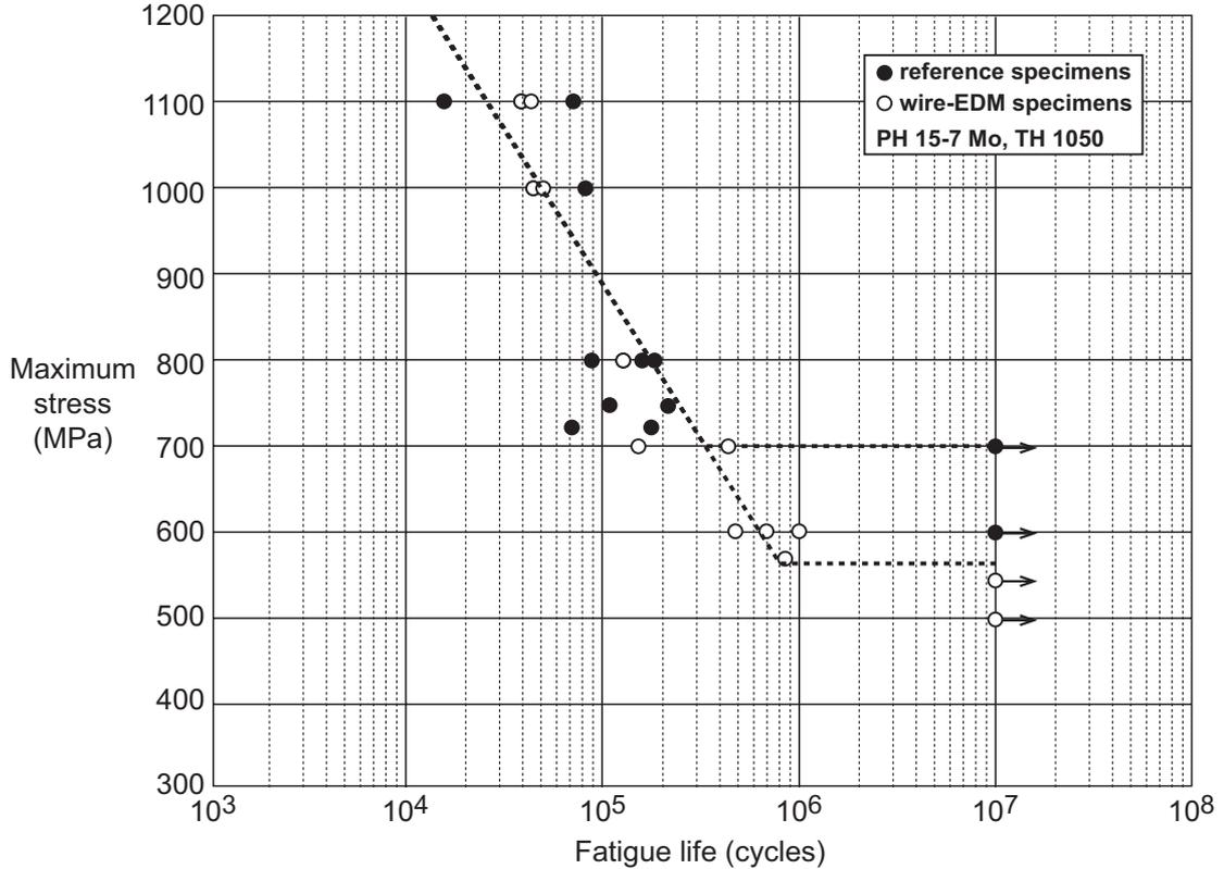
Fig. 5 Effect of wire-EDM on fatigue of PH 15-7 Mo stainless steel (reference specimens were abrasive jet machined,  $K_t = 1.06$ ,  $R = 0.1$ : see subsection 1.5.2)
