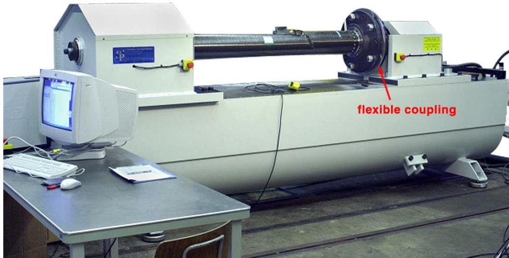
**Fig. 10** Torsional fatigue testing of filament wound carbon/epoxy - metal flange drive shafts
