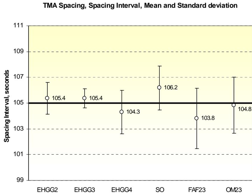
Figure 19: Relative spacing (in time) over waypoints.
