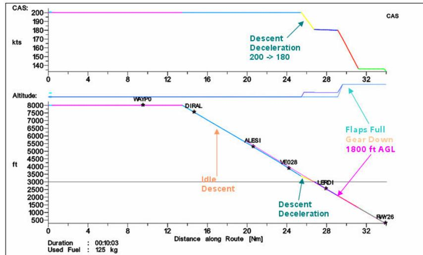
Figure 6: ACDA for the ATTAS VFW614 aircraft.
