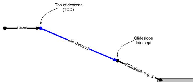
Figure 4: Generic vertical profile of an ACDA.
