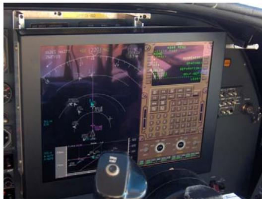
*Figure 14: Display layout with temporary CDU.*
