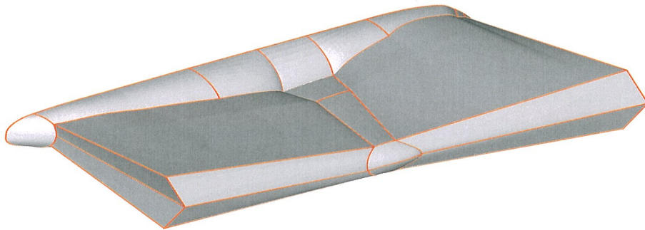
Fig. 1(b) Domain decomposition around the DLR-F4 wing body configuration using the domain modeler ENDOMO, part of the ENFLOW CFD system: the first layer of blocks around the configuration plus the additional blocks to make this layer more convex, as needed for the 'potential' method. Red lines indicate the block boundaries.
