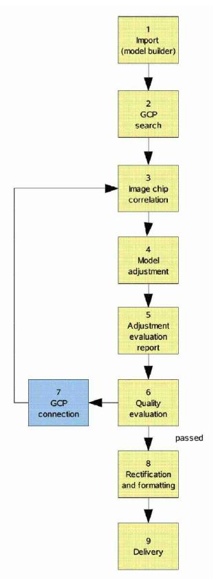
Fig. 4 Flow diagram for automatic ortho-rectification
