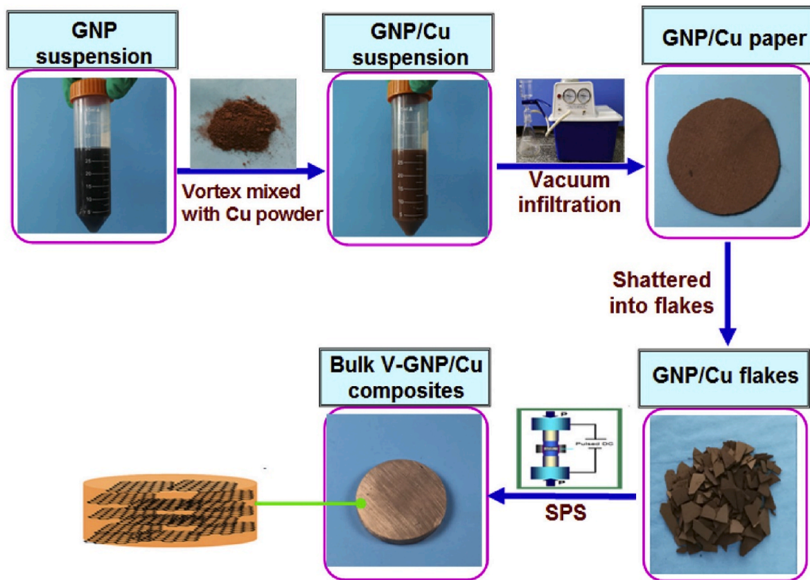
Fig. 17. Enhancing the copper powder with GNP suspension [49].
