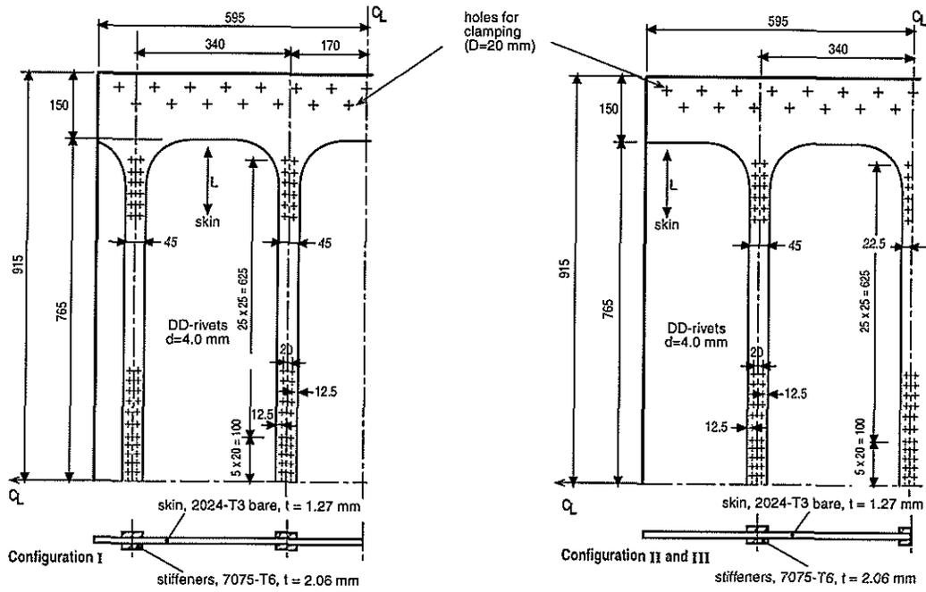
Figure 1 Panel design uncracked
