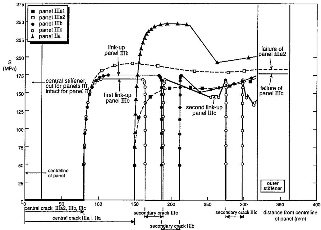
Figure 4 Crack growth curve for panel types II and III
