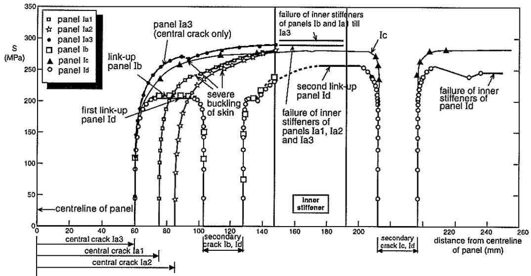
Figure 3 Crack growth curve for panels I
