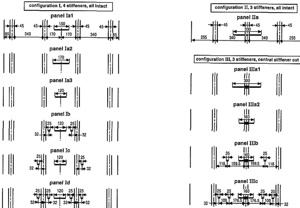
Figure 2 Crack configurations as machined
