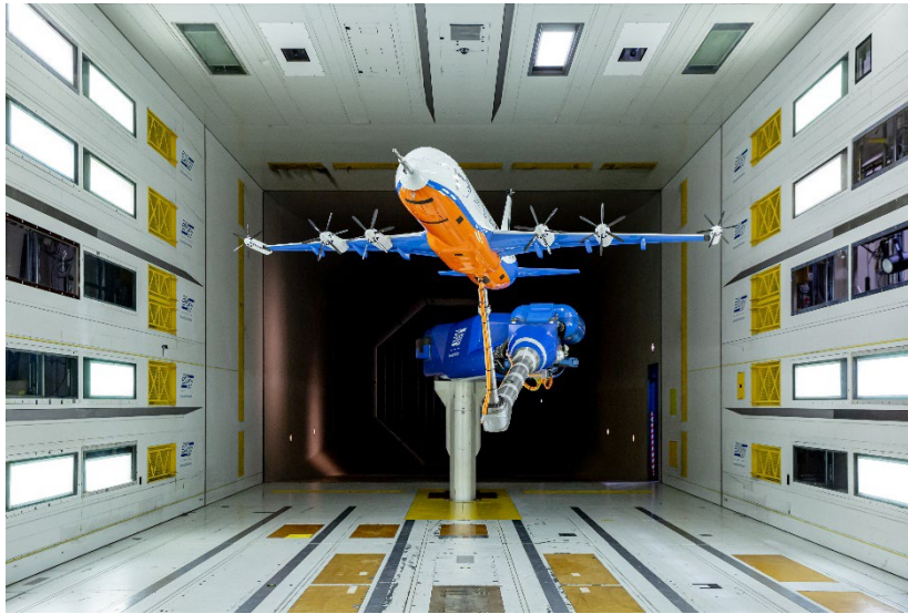
Figure 2 DEP-SFD in the DNW wind tunnel
