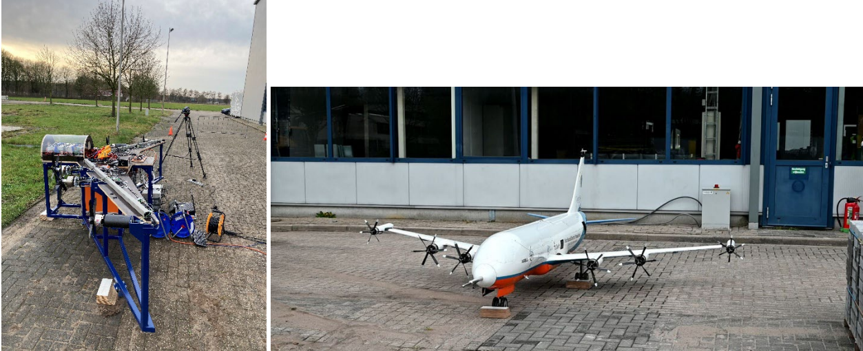
Figure 3 Iron bird test facility and the DEP-SFD on chocks during a stationary test
