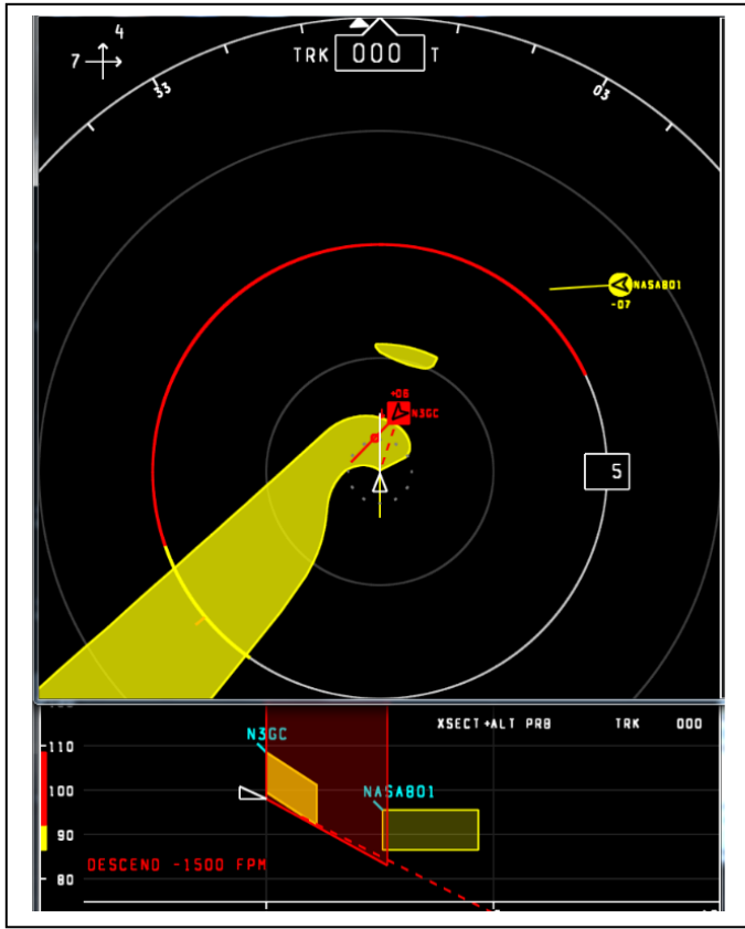
Fig. 2. Example CPDS display with DWC and TCAS RA guidance.
