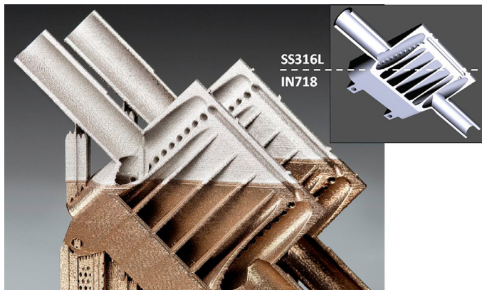
Fig. 7. Multi-material heat exchanger functionally graded from IN718 (bottom) to SS316L (top) shown after homogenization heat treatment.
