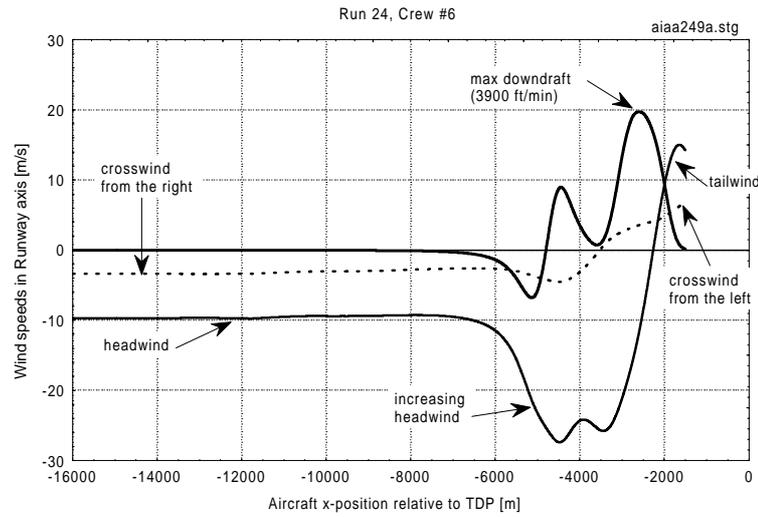
Fig. 27 Wind speeds versus distance for crew 6 on run 24.
