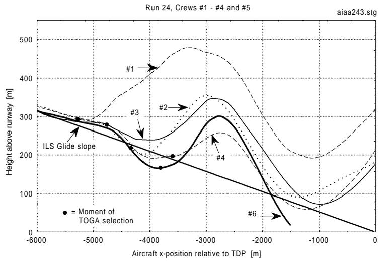
Fig. 25 Detail of height versus path along the ILS glide slope (crew 5 left out).
