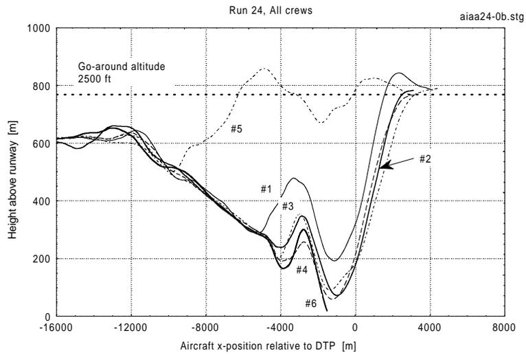
Fig. 24 Height versus distance path for all crews.
