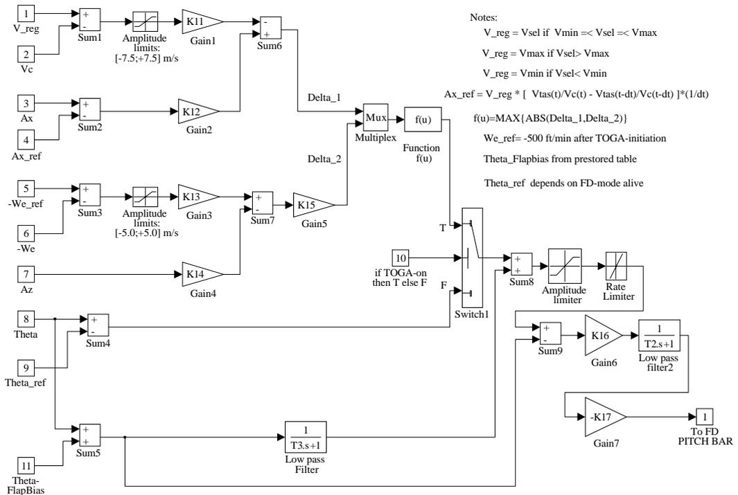
Fig. 2 Flight director standard (STD) pitch steering mode for the go-around.
