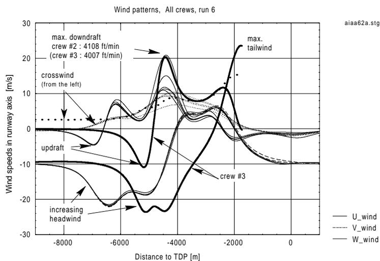
Fig. 20 Wind speeds encountered along the trajectory for all crews.
