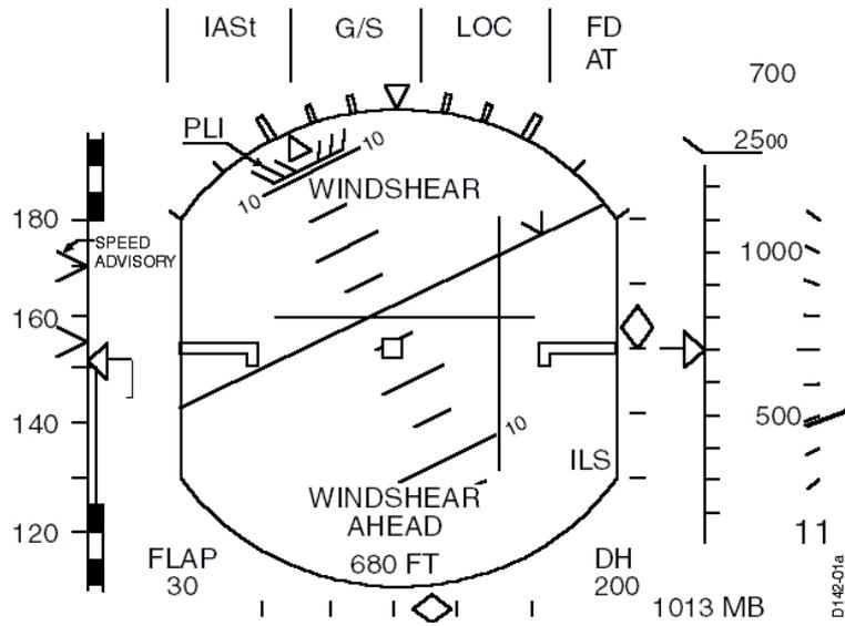
Fig. 1 EFIS/PFD showing windshear labels, the Pitch Limit Indicator (PLI) and the speed advisory.
