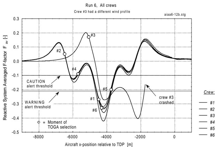
Fig. 19 Averaged F-factor of the reactive system as function of distance from touchdown.
