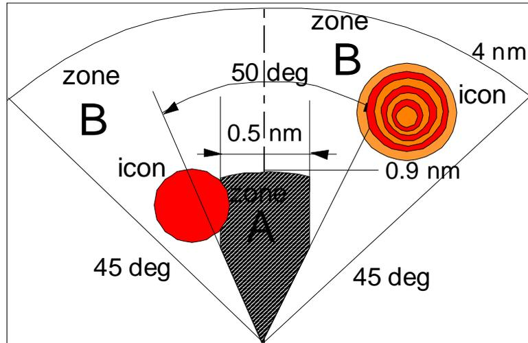
Fig. 12 Hazard zone A and B (relative to aircraft's longitudinal axis) and a red and an amber/red colored windshear icon.
