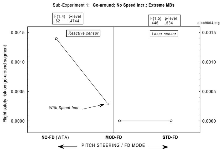
Fig. 9 Effect of pitch steering on flight safety risk in the go-around segment.
