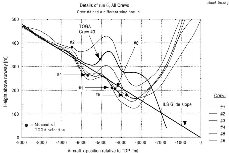
Fig. 18 Detail of height versus distance along the ILS glide slope and in the go-around.
