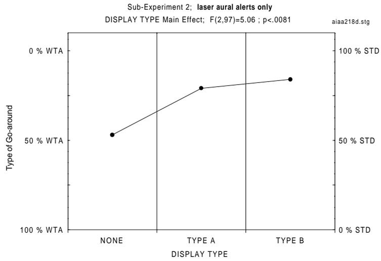
Fig. 16 Type of go-around as function of display type.
