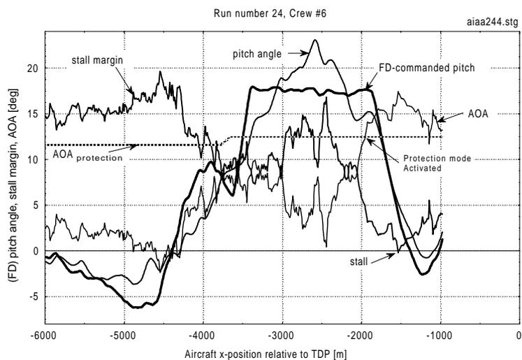
Fig. 28 Pitch angle, FD-commanded pitch, AOA and stall margin for crew 6 on run 24.
