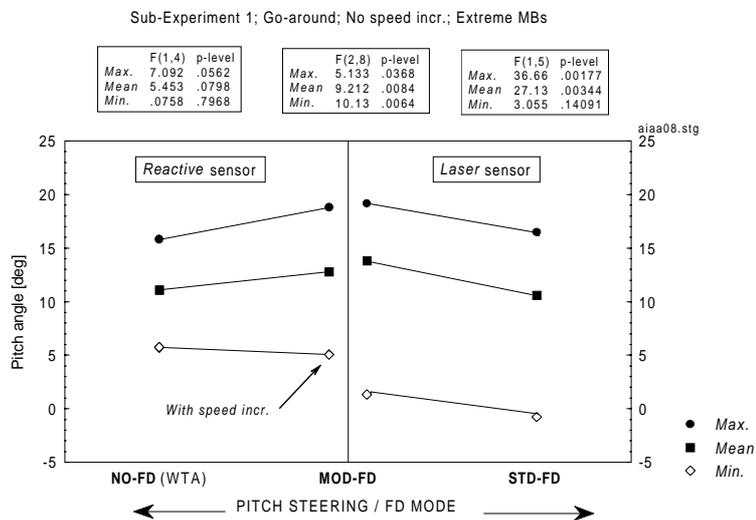
Fig. 7 Effect of pitch steering (FD-mode) on pitch angle in the go-around.
