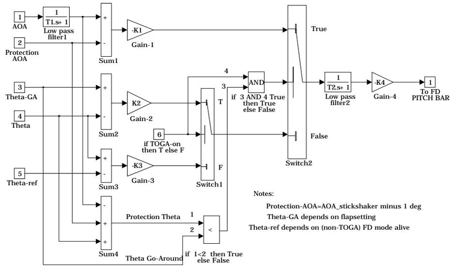
Fig. 3 Flight director MODified (fixed) pitch mode with angle of attack protection.
