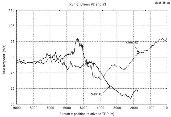
Fig. 22 True airspeed along the trajectory for crews 2 and 3.
