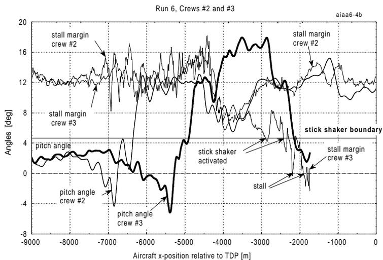
Fig. 21 Pitch angle and angle of attack time histories along the trajectory for crews 2 and 3.
