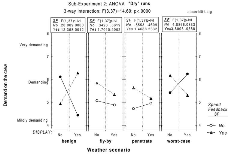
Fig. 14 Effect of icon display on crew workload per weather scenario, as function of speed feedback.
