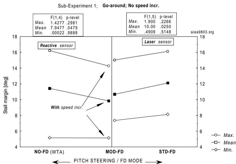
Fig. 6 Effect of pitch steering on the stall margin in the go-around.
