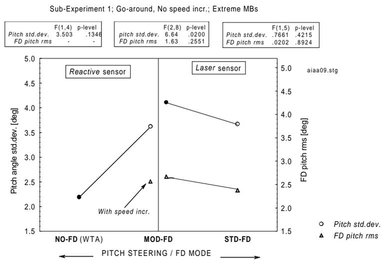
Fig. 8 Effect of pitch steering (FD-mode) on the pitch angle standard deviation and the FD rms.
