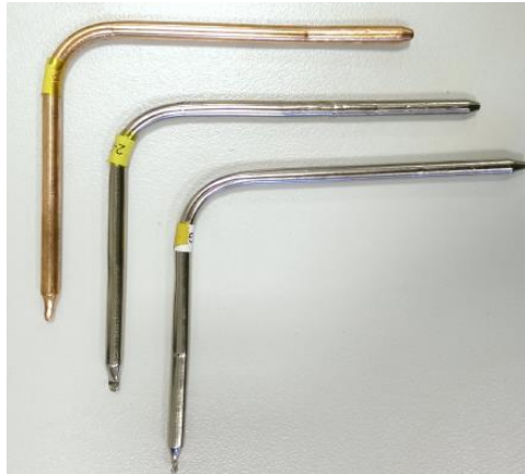
Figure 19. Photo of 3 bended heat pipes.
