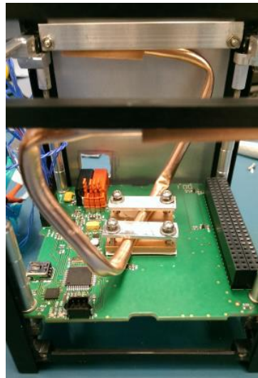
Figure 20. Photo of a CubeSat (with some panels removed) with a heat pipe.
