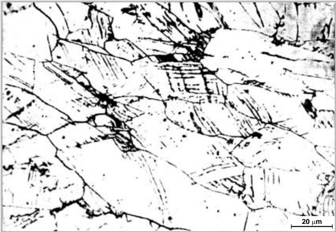
Corrosion along slip lines, possibly also along deformation twin boundaries, and intergranular cracks: metallograph (Thompson and Chatterjee 1954)
