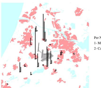
Per NMT, bar no.; 1- Measured NA70 2- Calculated NA70
