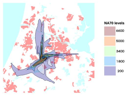
Figure 1: Grid NA70 calculation for June 2003 07h-19h
