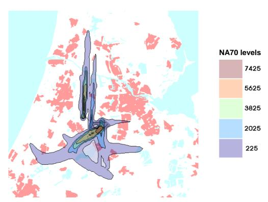
Figure 3: Grid NA70 calculation for November 2003 07h- 19h
