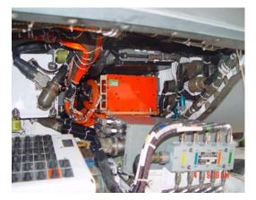
Figure 8 PMU in Aft avionics compartment
