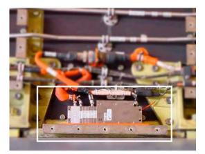
Figure 7 Remote unit at RH side of vertical tail
