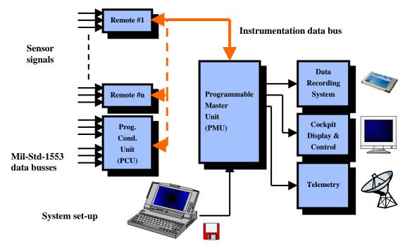
Figure 6 Schematic overview of the Instrumentation System (single recorder PCM/Audio configuration)
