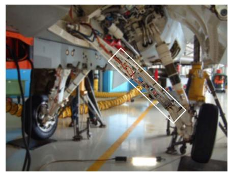
Figure 11 Instrumented landing gear, left lower drag brace is TMC (in the box)
