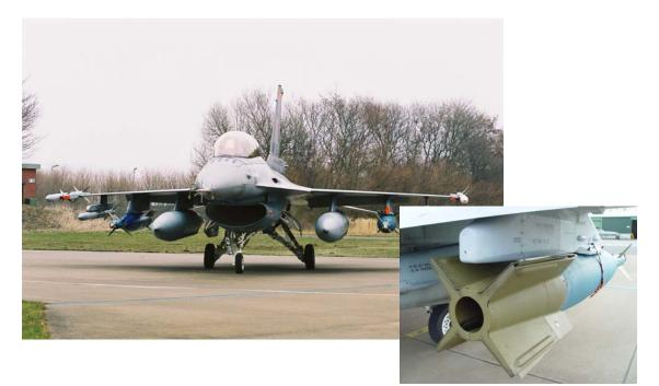
Figure 10 Instrumented GBU10 mounted under PIDS at STA3&7
