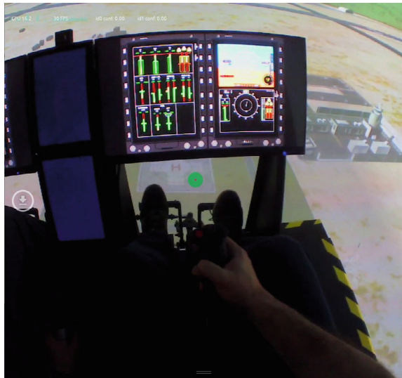
Fig. 13.7 Post engine failure eye tracking during the descent phase of the FTM
