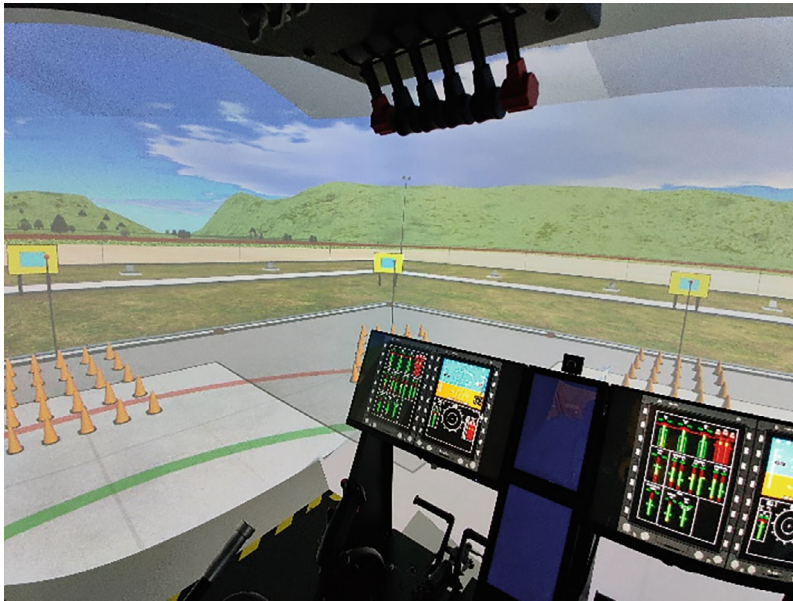
Fig. 12.5 Cockpit view of X-Wind Hover (XWH) low-speed controllability ACR simulator set-up in UoL's HELIFLIGHT-R simulator [21]
