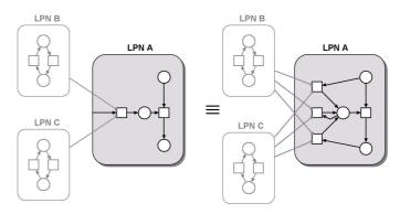
FIGURE 10.3: High level ordinary arc starts on the edge of an LPN box and ends on a transition inside the same LPN box.
