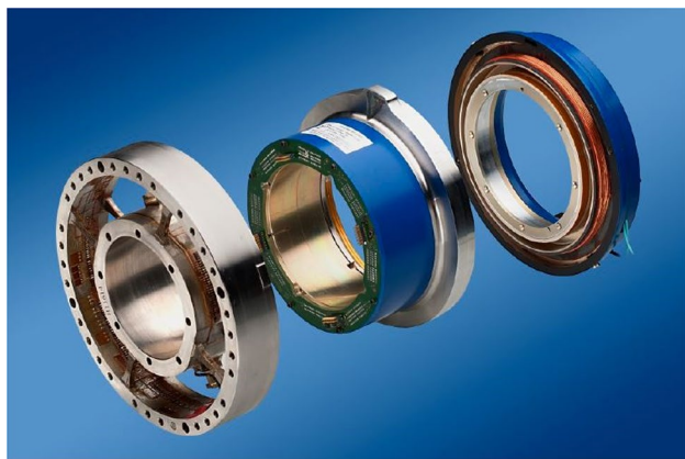
Fig. 1 Example of an NLR rotating shaft balance (left) with telemetry rotor (mid) and stator (right) [1]
