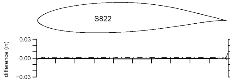
Figure 7-2: S822 airfoil model accuracy (difference between specified and measured coordinates).
