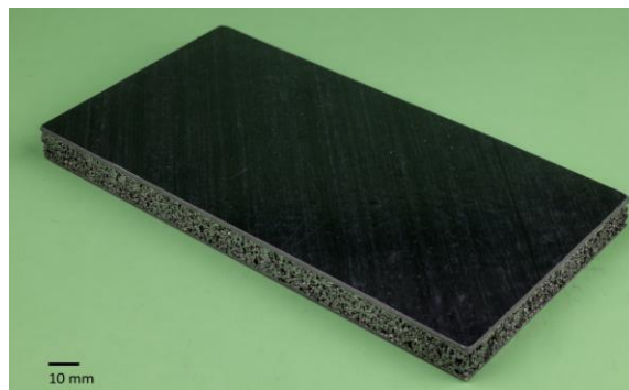
Fig. 1. Sandwich panel with carbon foam core and carbon fibre reinforced polyaryletherketone facing.
