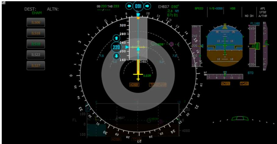
Figure 8. Interaction screen for speed and heading adjustments
