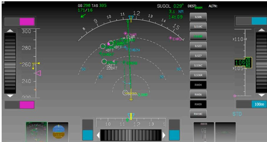
Figure 2. HMI design phase 1 using touch wheels
