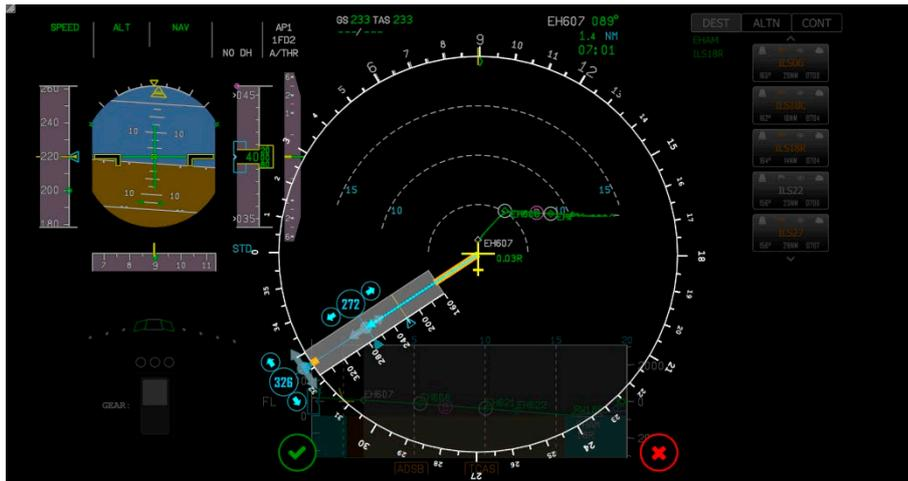
Figure 14. Interaction screen for decoupled speed and heading adjustments
