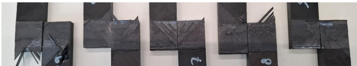
Figure 11: Fracture surfaces of the welded samples
