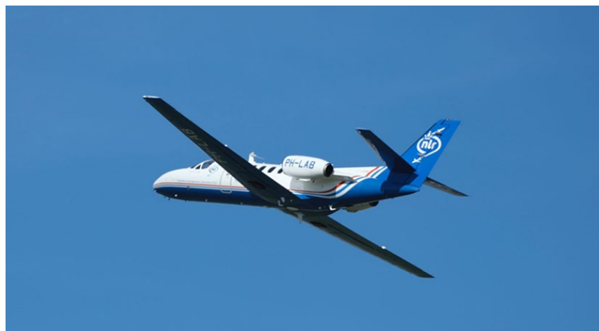
Figure 1 NLR Cessna Citation II flight inspection aircraft equipped with Garmin/Aerodata Flight Inspection System
