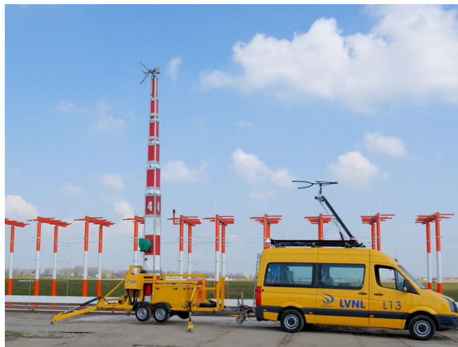
Figure 2 LVNL measurement car with LOC antenna on top, and towing a lorry with extensible mast having on top the receiving GP antenna.
