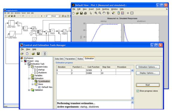
Figure 9: Screenshot of engine startup/shutdown optimization in Matlab-Simulink
