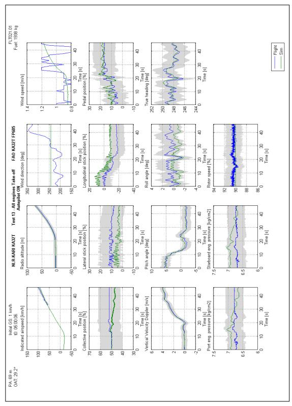
Figure 10: Example of comparison between model and flight test data for the take-off maneuver
