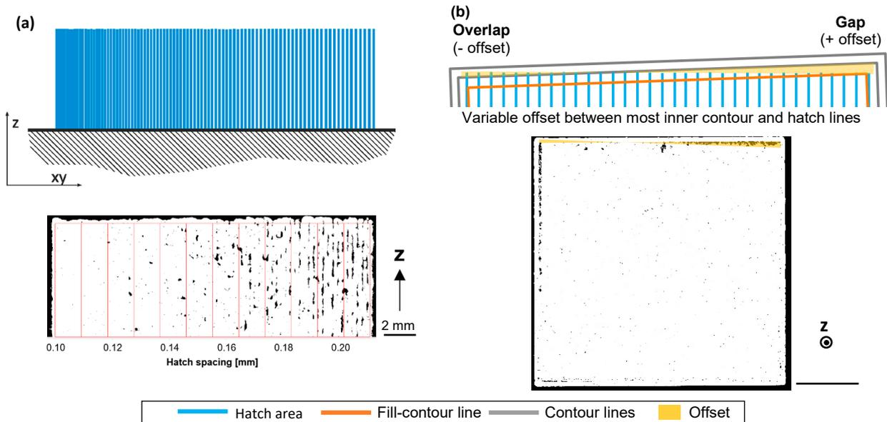
Figure 1 (a) Example of a block with variable hatch distance across the length, where the 12 analysed fields are depicted with red colour rectangles. (b) Schematic representation of the blocks built with a rotated hatch for creating a variable offset along the edge.
