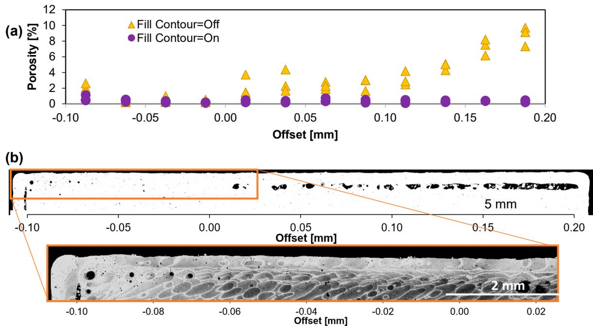
Figure 4 Evaluation of the contour hatch interface with a variable offset along the length. (a) Porosity percentage as a function of the offset for the blocks built without fill-contour and with fill-contour. (b) Block without fill-contour showing a good overlap for offsets < 0.00 mm.
