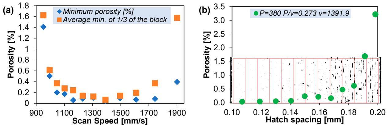
Figure 3 (a) Minimum porosity in one field and in four fields as function of the scan speed, for samples built with 380 W. (b) Porosity percentage of the chosen block for the hatch spacing (380 W and 1392 mm/s).
