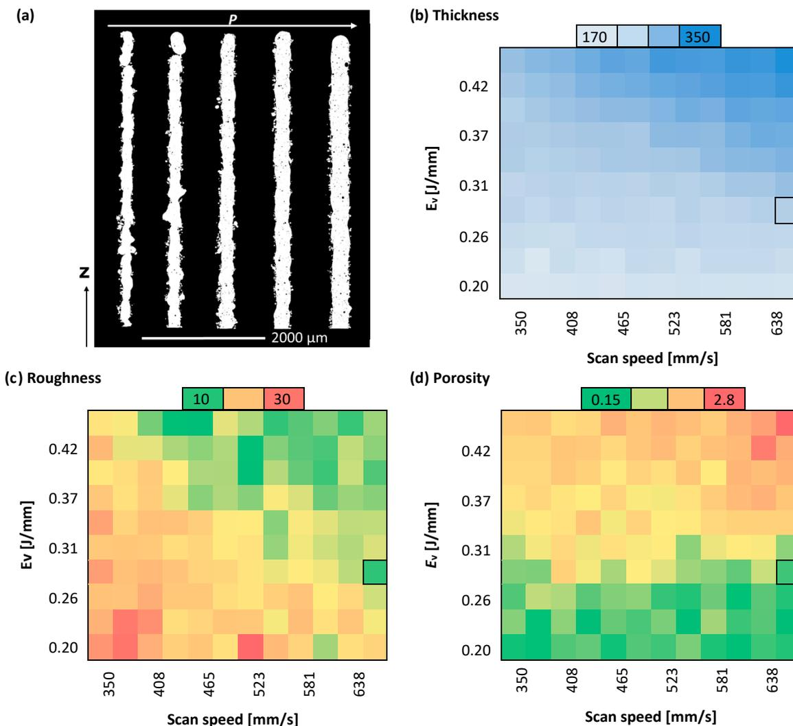
Figure 2 Evaluation of the thin walls based on the (a) cross-sections. In (a), several walls are shown built with 494 mm/s and increasing laser power from left to right. (b) Thickness, (c) porosity and (d) roughness of the walls as a function of the scan speed and linear energy density ( $E_v$ ).
