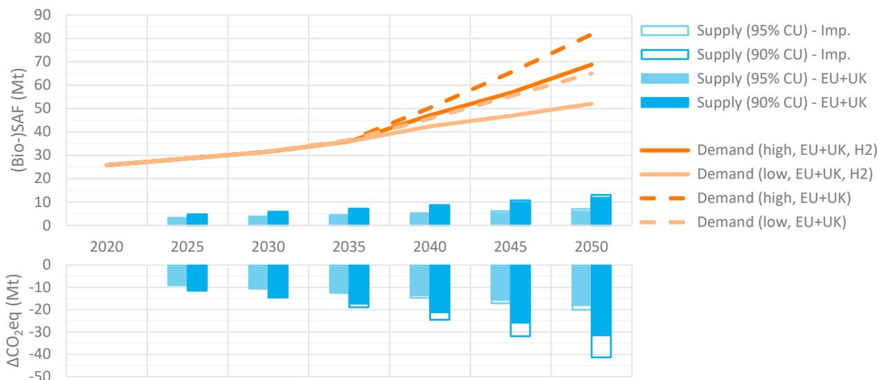
Figure 18: Bio- or waste-based SAF supply from Fischer-Tropsch production and total SAF demand (top) and associated net CO<sub>2</sub>eq emissions reduction (bottom) in different traffic scenarios and cases of competing use of biomass (CU) with supply from EU + UK only or with additional import from selected non-European production (Imp.)
