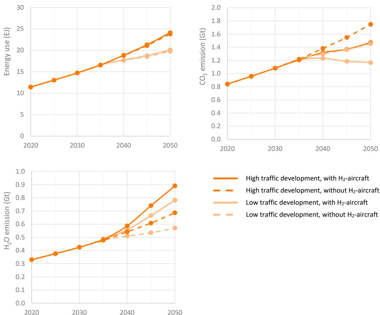
Figure 2: Global aircraft energy use and gross emissions at fleet level in **high** or **low** traffic scenarios, both with (solid lines) and without (dashed lines) hydrogen-powered aircraft in the fleet
