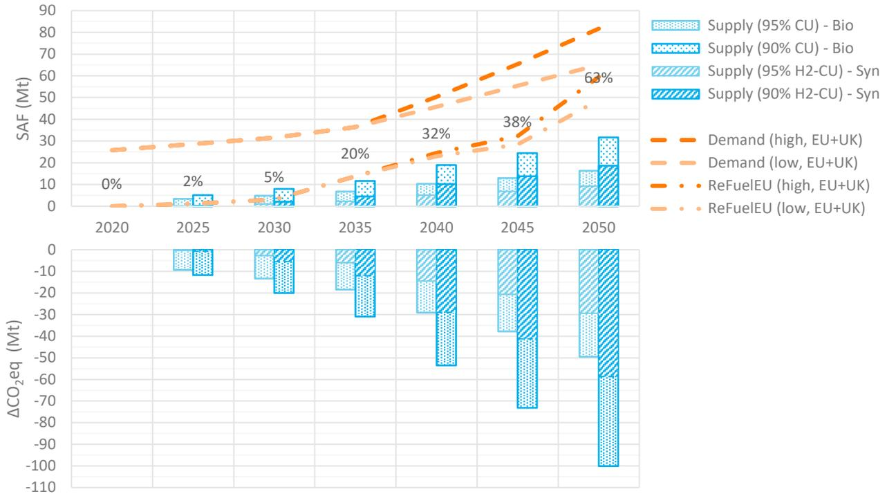
Figure 43: Total SAF supply and SAF demand (based on fleet-based blending limits or indicated ReFuelEU Aviation mandate; top) and net CO<sub>2</sub>eq emissions reduction (bottom) in different traffic scenarios (without hydrogen-powered aircraft) and cases of competing use with EU, UK and imported supply
