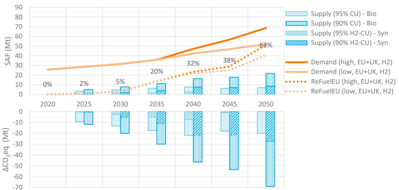
Figure 22: Total SAF supply (bio- or waste-based Fischer-Tropsch and synthetic) and SAF demand (based on fleet-based blending limits or ReFuelEU Aviation mandate<sup>22</sup> as numerically indicated; top) and net CO<sub>2</sub>eq emissions reduction (bottom) in different traffic scenarios (with hydrogen-powered aircraft) and cases of biomass and hydrogen competing use (CU) with EU, UK and imported supply
