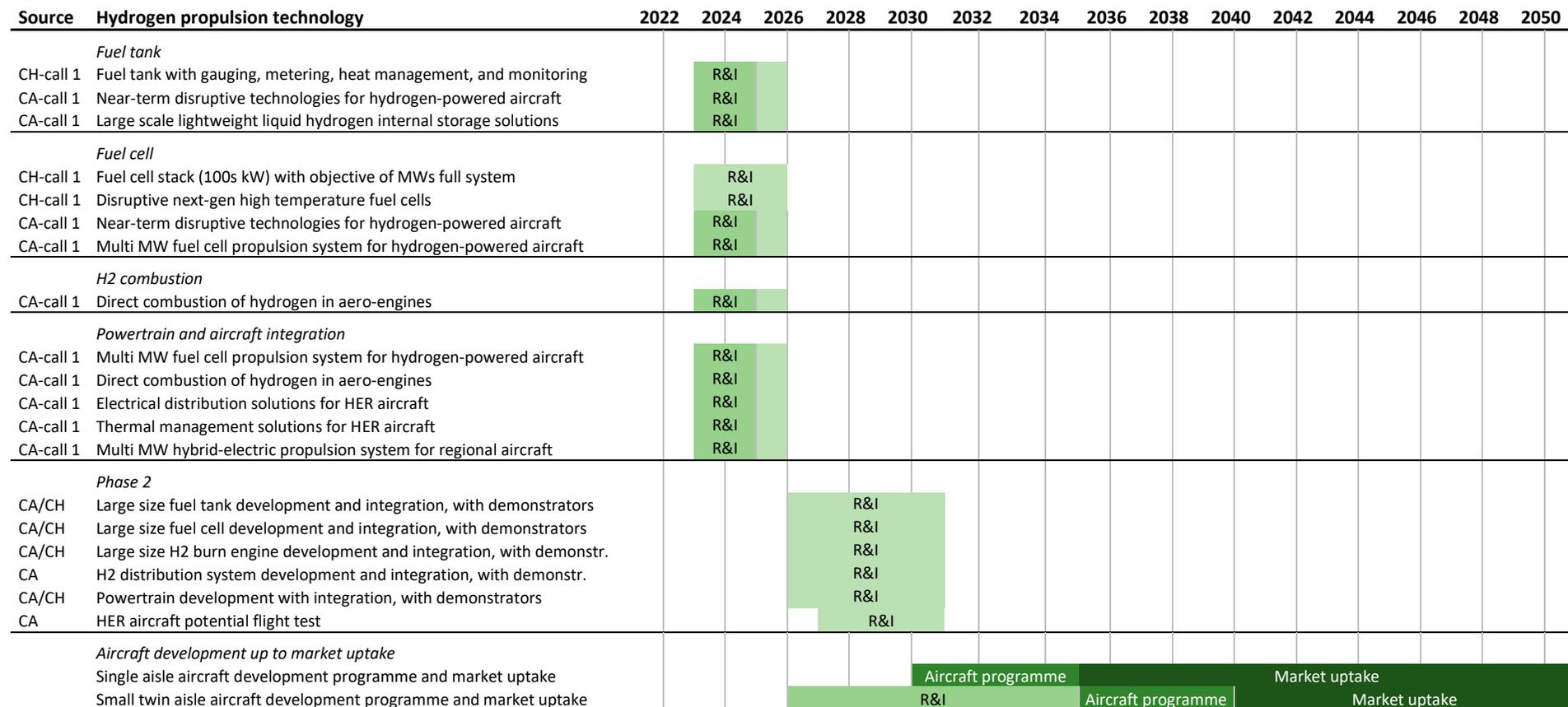
Figure 13: European roadmap for hydrogen-powered propulsion (based on Clean Aviation, 2021; Clean Aviation Joint Undertaking, 2022; Hydrogen Europe and Hydrogen Europe Research, 2020). CA is Clean Aviation, CH is Clean Hydrogen, R&I is research and innovation. The lightest green indicates scheduling uncertainty
