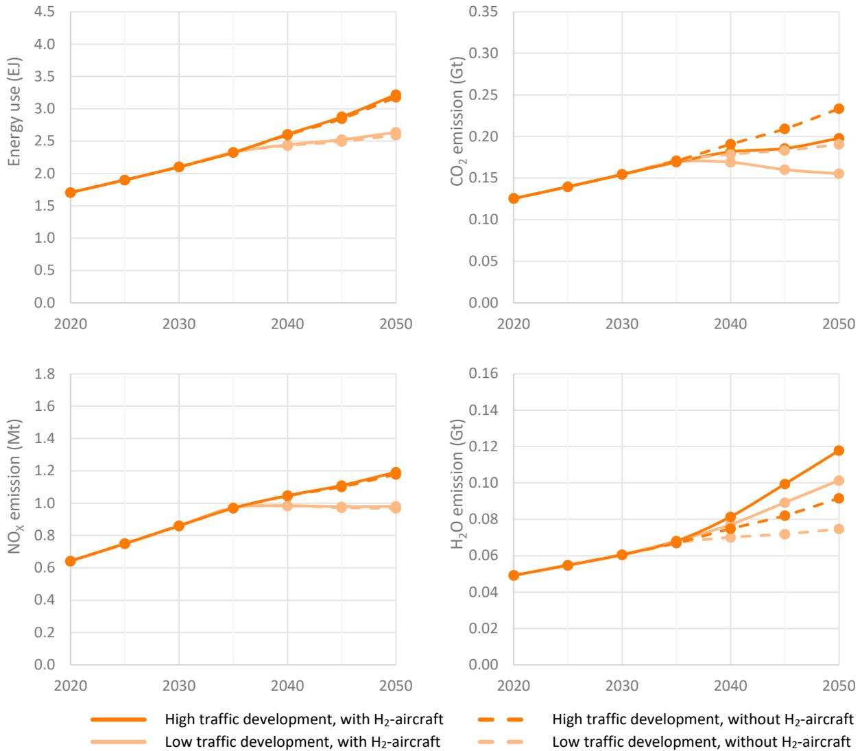
Figure 36: Aircraft energy use and emissions by aircraft departing from EU27 airports under **high** or **low** traffic development, and with (solid lines) or without (dashed lines) hydrogen-powered aircraft
