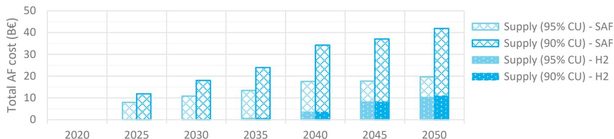
Figure 25: Total annual cost of alternative fuels supplied from EU, UK and imported production in traffic scenario with hydrogen-powered aircraft and different cases of competing use (CU) in billions of Euros
