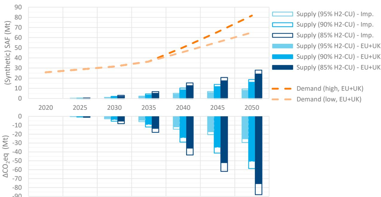
Figure 41: Synthetic SAF supply and total SAF demand (top) and associated net CO<sub>2</sub>eq emissions reduction (bottom) in different traffic scenarios (without hydrogen-powered aircraft) and cases of competing use with supply from EU + UK only or with additional import from selected non-European production (Imp).
