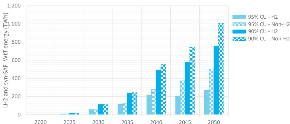
Figure 48: Total well-to-tank energy requirements for production of available LH<sub>2</sub> and synthetic SAF in scenarios with and without hydrogen-powered aircraft and different cases of competing use with EU, UK and imported supply
