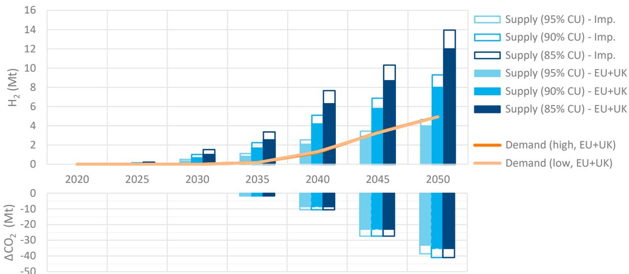
Figure 15: Hydrogen supply and demand (top; almost identical between low and high traffic scenarios) and gross CO<sub>2</sub> emissions reduction (bottom) in different traffic scenarios and cases of hydrogen competing use (CU) with supply from EU + UK only or with additional import from selected non-European production (Imp.)
