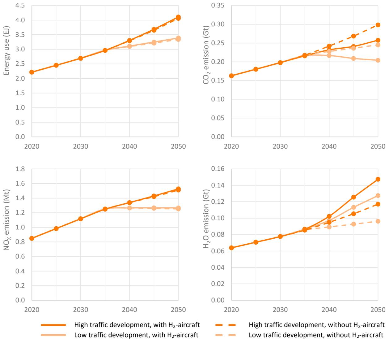
Figure 37: Aircraft energy use and emissions by aircraft departing from EU + UK airports under high or low traffic development, and with (solid lines) or without (dashed lines) hydrogen-powered aircraft
