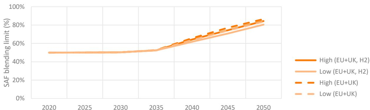
Figure 14: Fleet-based blending limit for SAF
