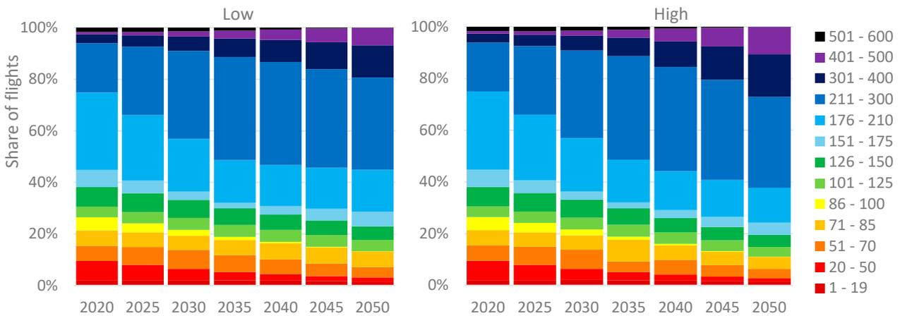
Figure 34: Fleet composition of flights departing from EU + UK, airports according to aircraft size class in the two traffic development scenarios considered
