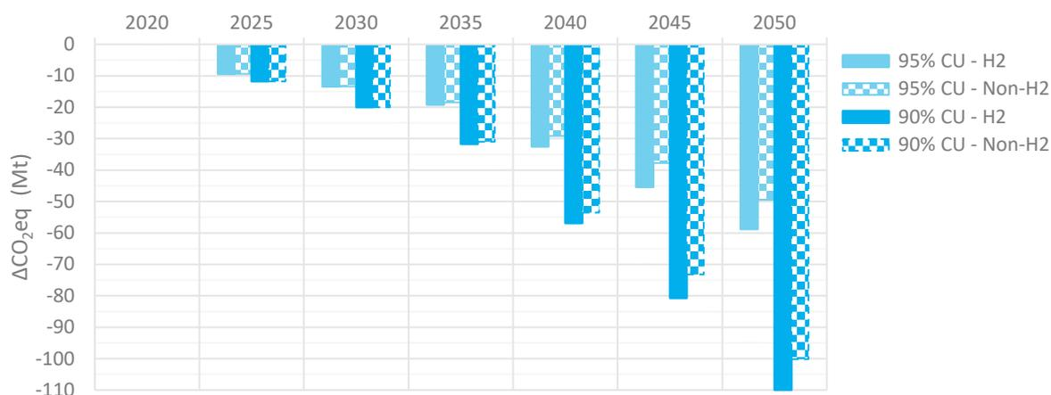
Figure 26: Total CO<sub>2</sub>(eq) emissions reduction realised in scenarios with and without hydrogen-powered aircraft and different cases of competing use (CU)
