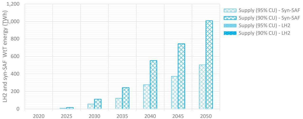
Figure 50: Total well-to-tank energy requirements for production of available LH<sub>2</sub> and synthetic SAF in a scenario without hydrogen-powered aircraft and different cases of competing use with EU, UK and imported supply
