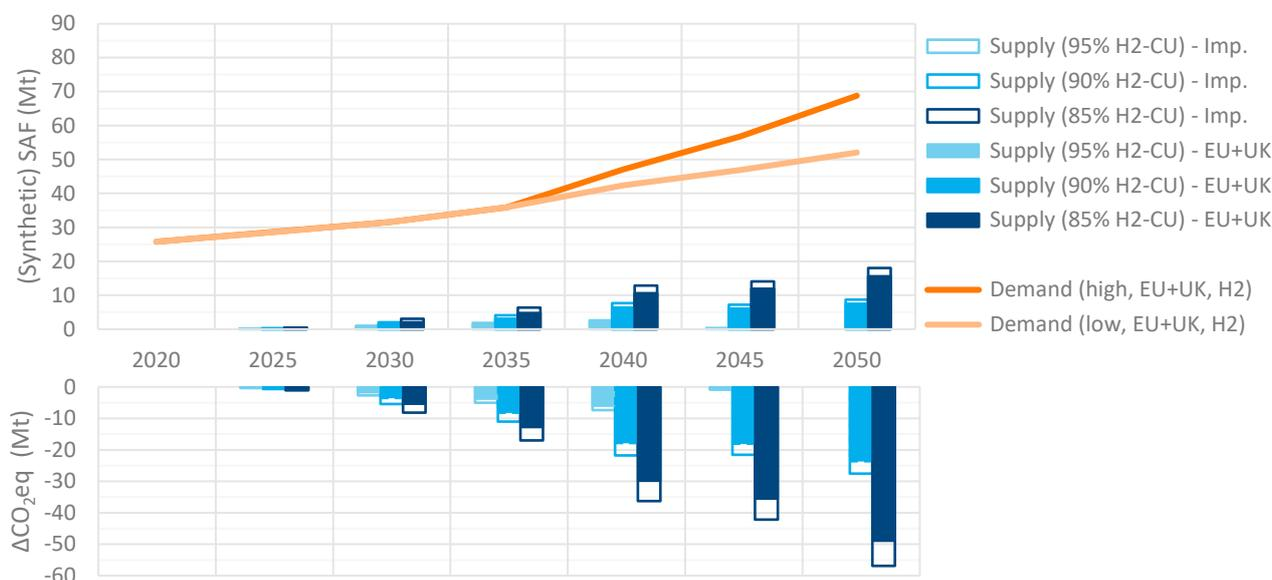
Figure 20: Synthetic SAF supply and total SAF demand (top) and associated net CO<sub>2</sub>eq emissions reduction (bottom) in different traffic scenarios (with hydrogen-powered aircraft) and cases of hydrogen competing use (CU) with supply from EU + UK only or with additional import from selected non-European production (Imp.)
