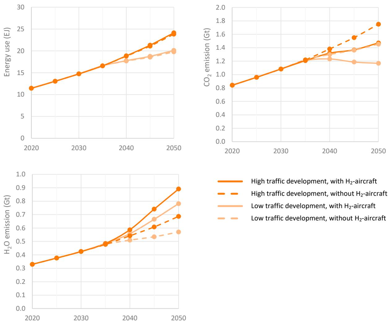
Figure 28: Global aircraft energy use and gross emissions at fleet level in **high** or **low** traffic scenarios, both with (solid lines) and without (dashed lines) hydrogen-powered aircraft in the fleet
