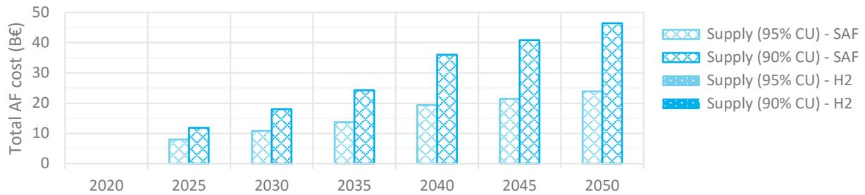
Figure 46: Total annual cost of alternative fuels supplied from EU, UK and imported production in traffic scenario without hydrogen-powered aircraft and different cases of competing use (in billions of Euros)
