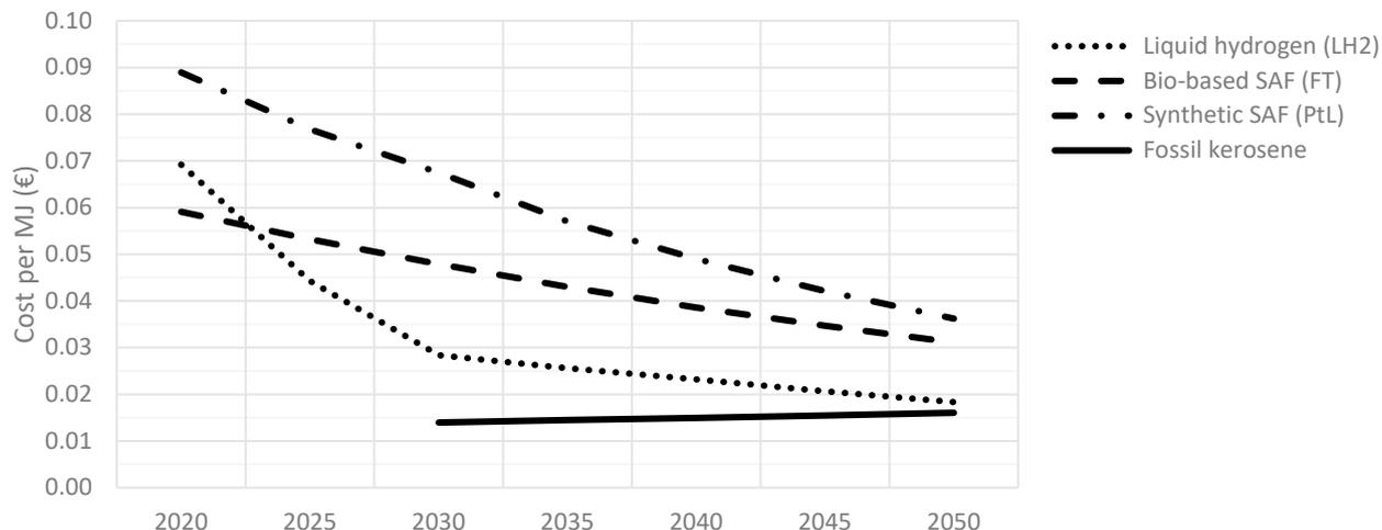
Figure 47: Cost of alternative fuels and fossil kerosene (€/MJ)
