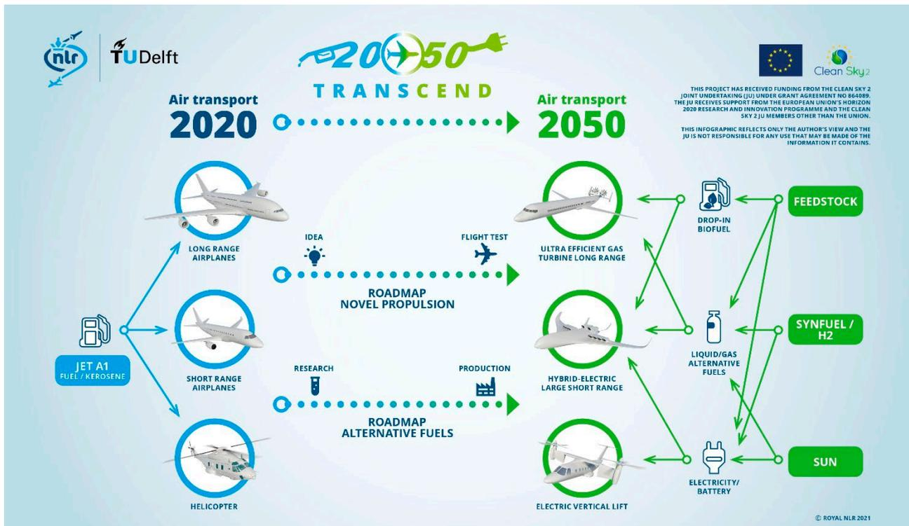
Figure 1: Infographic of the TRANSCEND project on the evaluation of the potential contribution of novel propulsion and alternative fuels to climate neutral aviation in 2050 and on roadmaps for novel propulsion and alternative fuels to achieve this potential contribution. The aircraft and fuels shown in 2050 indicate propulsion and fuels considered, not necessarily the propulsion and fuels that have been evaluated
