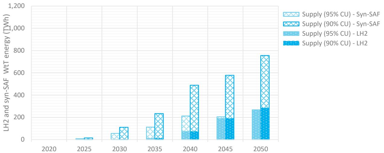
Figure 49: Total well-to-tank energy requirements for production of available LH<sub>2</sub> and synthetic SAF in a scenario with hydrogen-powered aircraft and different cases of competing use with EU, UK and imported supply
