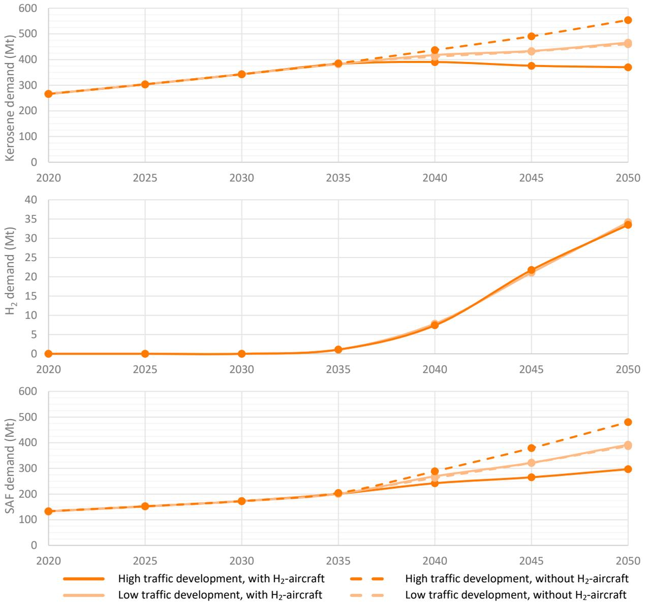
Figure 40: Global fuel demand (total kerosene, hydrogen and SAF) under **high** or **low** traffic development, and with (solid lines) or without (dashed lines) hydrogen-powered aircraft
