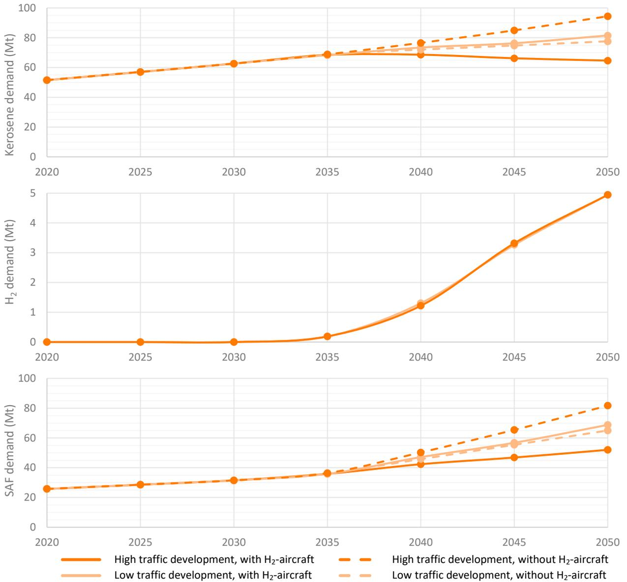
Figure 39: Fuel demand (total kerosene, hydrogen and SAF) by aircraft departing from EU + UK airports under high or low traffic development, and with (solid lines) or without (dashed lines) hydrogen-powered aircraft
