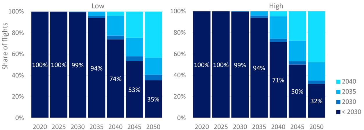
Figure 32: Fleet composition of flights departing from EU27 airports according to aircraft entry into service (EIS) year in the two traffic development scenarios considered (based on Gelhausen, Grimme, Junior, Lois, & Berster, 2022). Aircraft with EIS in 2030 or later are Clean Sky 2 aircraft
