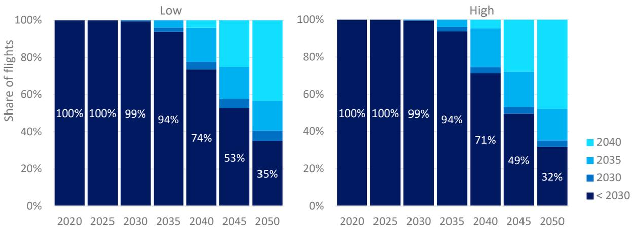
Figure 35: Fleet composition of flights departing from EU + UK airports according to aircraft entry into service (EIS) year in the two traffic development scenarios considered (based on Gelhausen, Grimme, Junior, Lois, & Berster, 2022). Aircraft with EIS in 2030 or later are Clean Sky 2 aircraft
