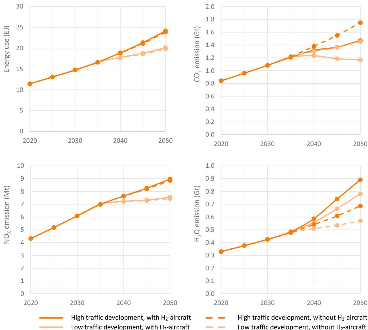
Figure 11: Global aircraft energy use and emissions under high or low traffic development, and with (solid lines) or without (dashed lines) hydrogen-powered aircraft
