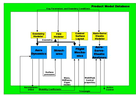
Figure 3 Preliminary CDE architecture for the global objective evaluation.
