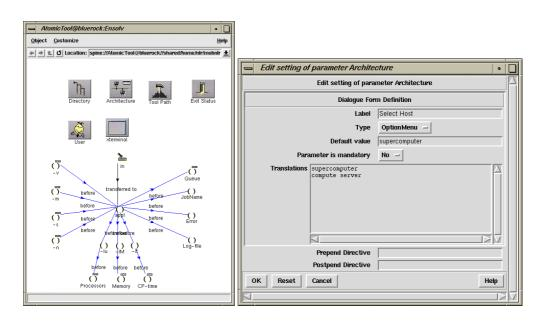
Figure 5 Examples of SPINEware AtomicTool editor windows. On the left the main editor window for the Ensolv CFD solver is given, where the icons represent AtomicTool sub-objects. On the right the sub-object Architecture-window for specification of the execution host is given.
