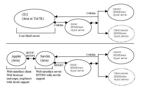
Figure 2 Two different ways of operation of the SPINEware user shell.
