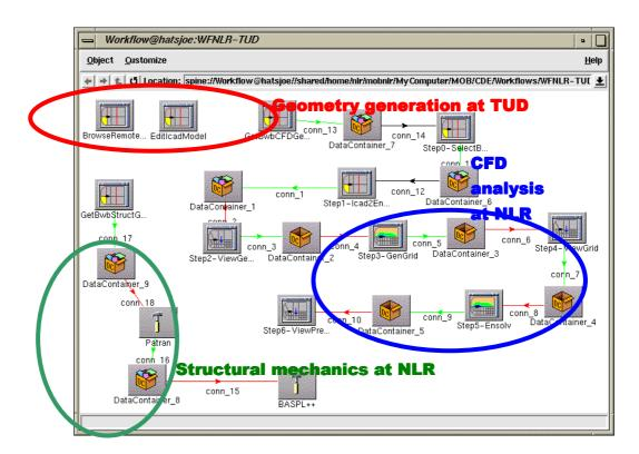
Figure 6 SPINEware WorkFlow object of the distributed BWB geometry generation and CFD and structural mechanics analysis processes, executed at the MOB partners TUD and NLR.
