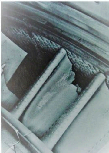
Broken and damaged 1 st stage turbine blades in civil aircraft engine
