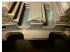
PHOTO 28: CLOSE-UP OF HPT STAGE 2 DISK LUG FRACTURE PHOTOS COURTESY OF IAE
