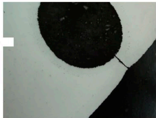
Crack initiation at location where film cooling hole intersects blade wall
