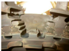
PHOTO 27: HPT STAGE 2 RELEASED BLADES AND DISK LUG FRACTURE
