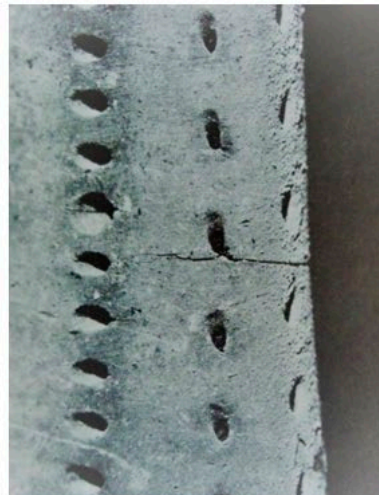
Detail of crack formation in leading edge of 1 st stage turbine blade
