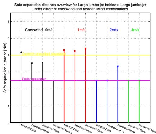
Figure 5.9 Safe separation distance for a Large Jumbo Jet behind Large Jumbo Jet
