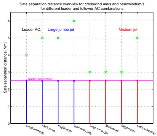
Figure E.4 Safe separation distance for a crosswind of 4 m/s
