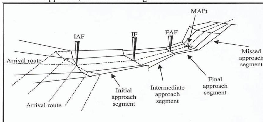
Figure 2.1 Instrument approach segments
