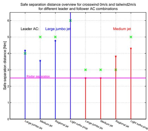
Figure F.2 Safe separation distance for a tailwind of 2 m/s and no crosswind
