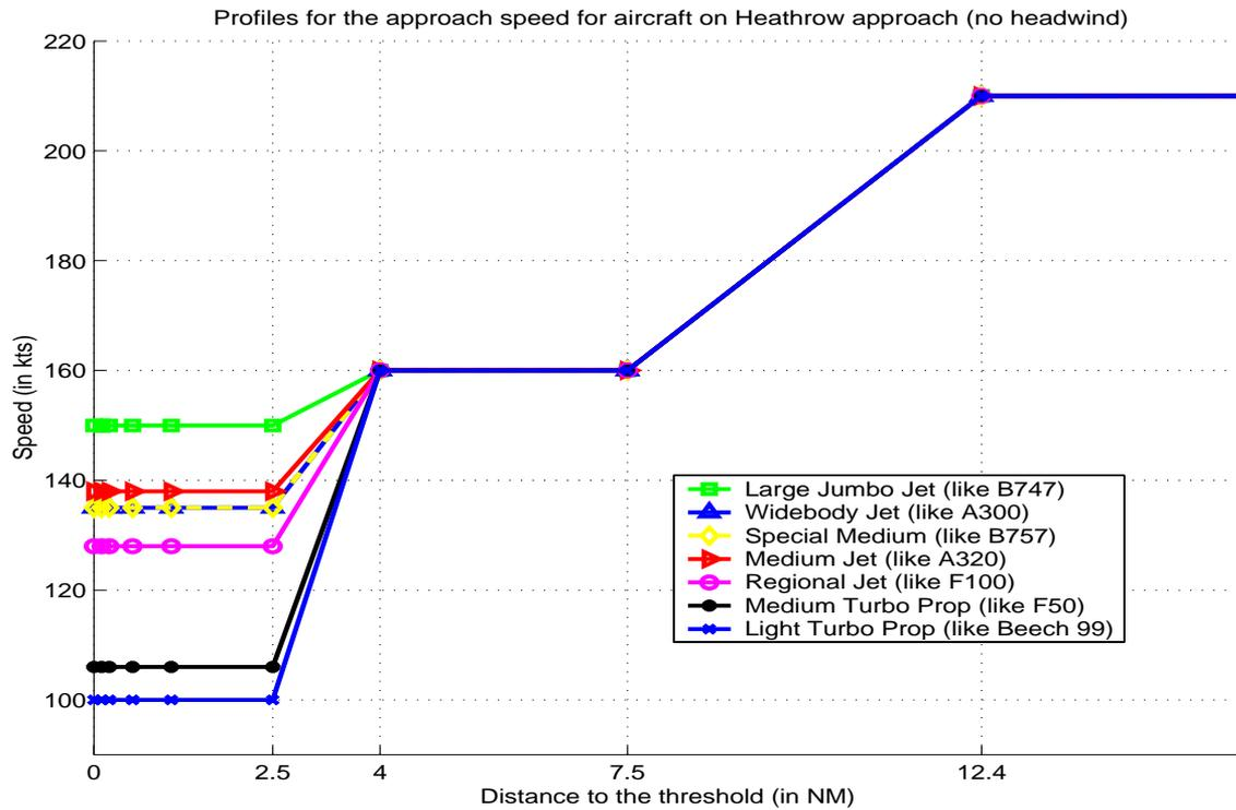
Figure 4.3 Speed profiles for aircraft on Heathrow approach
