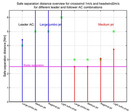
Figure 5.16 Safe separation distance for a crosswind of 1 m/s and a headwind of 2 m/s
