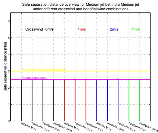
Figure C.2 Safe separation distance for a Medium Jet behind Medium Jet
