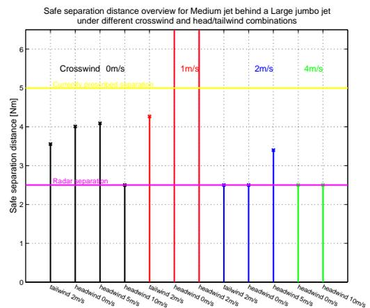
Figure 5.10 Safe separation distance for a Medium Jet behind Large Jumbo Jet
