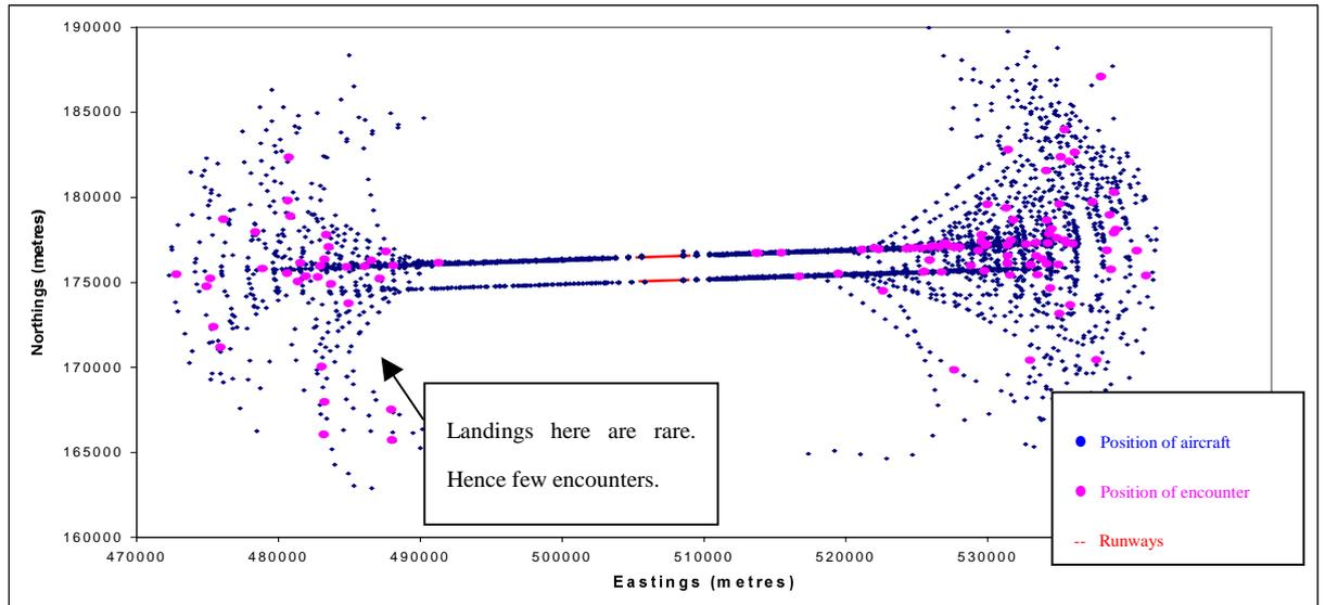
Fig. 5.19: Plan view of the London Heathrow area, with radar flight tracking and WVE positions detected by NLR-VORTEX from FDR data (preliminary result)
