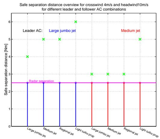
Figure G.4 Safe separation distance for a crosswind of 4 m/s and headwind of 10 m/s
