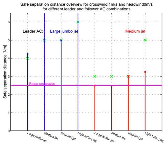
Figure E.2 Safe separation distance for a small crosswind of 1 m/s
