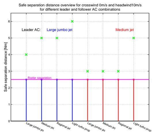
Figure 5.18 Safe separation distance for a headwind of 10 m/s and no crosswinds
