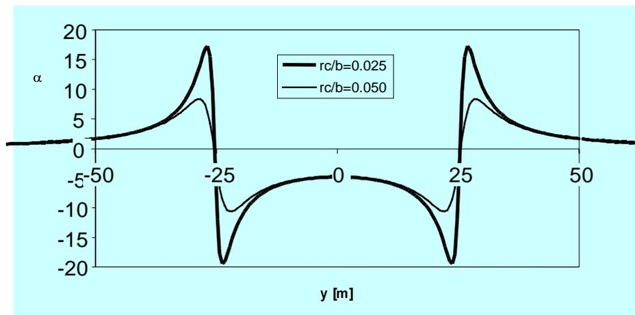
Figure 4.2 – Typical flow angles in the wake of a B747-400 aircraft on final approach for two typical vortex core sizes ( $rc$  is the vortex core size and  $b$  is the wing span)
