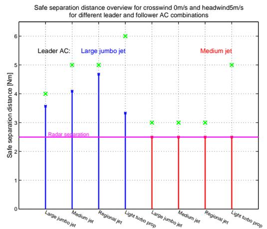
Figure D.3 Safe separation distance for a headwind of 5 m/s and no crosswind
