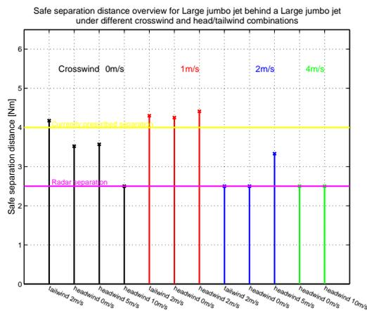
Figure B.1 Safe separation distance for a Large Jumbo Jet behind Large Jumbo Jet
