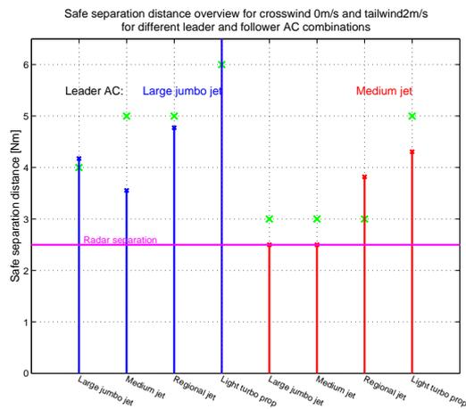
Figure D.1 Safe separation distance for a small tailwind of 2 m/s and no crosswind
