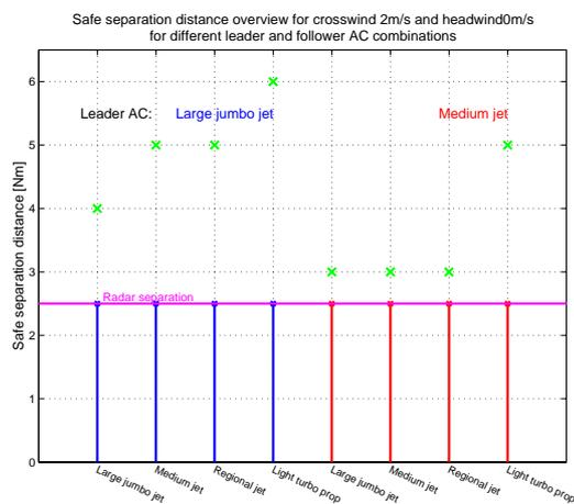
Figure 5.17 Safe separation distance for a crosswind of 2 m/s
