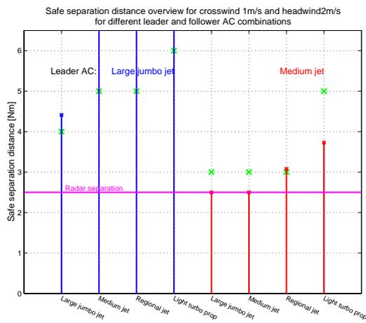
Figure G.2 Safe separation distance for a crosswind of 1 m/s and a headwind of 2 m/s
