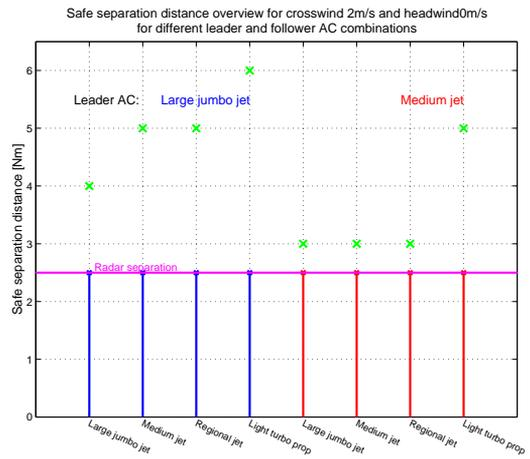
Figure E.3 Safe separation distance for a crosswind of 2 m/s
