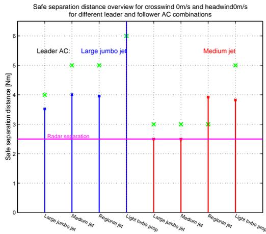
Figure E.1 Safe separation distance for the situation without wind conditions
