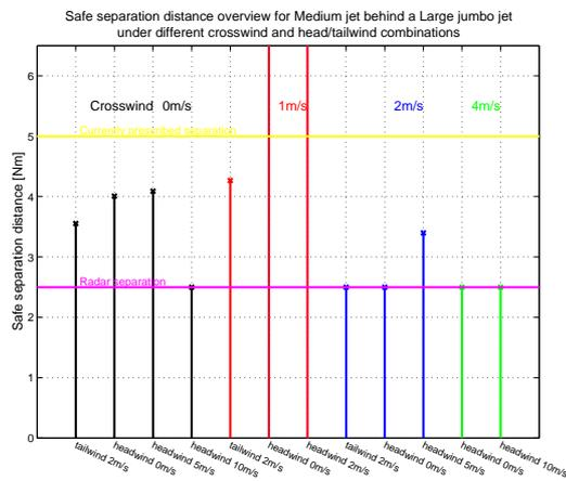
Figure B.2 Safe separation distance for a Medium Jet behind Large Jumbo Jet
