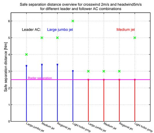
Figure G.3 Safe separation distance for a crosswind of 2 m/s and a headwind of 5 m/s
