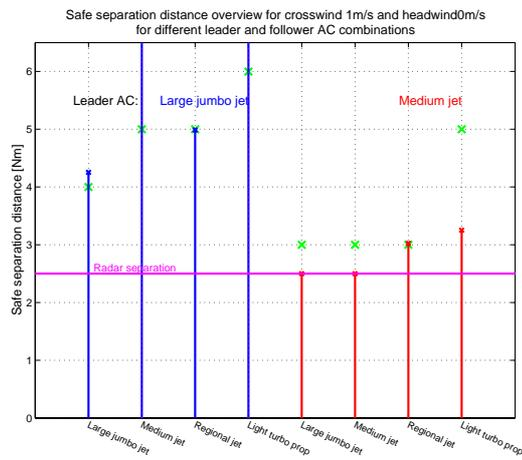
Figure 5.15 Safe separation distance for a small crosswind of 1 m/s
