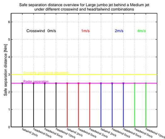
Figure C.1 Safe separation distance for a Large Jumbo Jet behind Medium Jet
