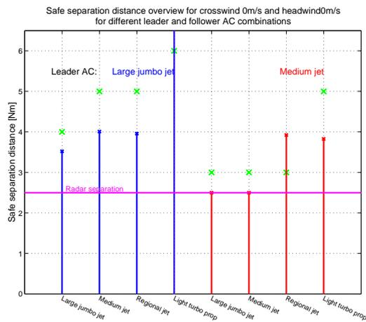
Figure F.1 Safe separation distance for the situation without wind conditions
