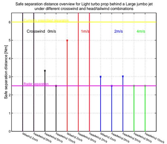
Figure 5.12 Safe separation distance for a Light Turbo Prop behind Large Jumbo Jet
