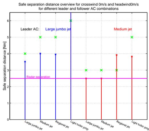
Figure G.1 Safe separation distance for the situation without wind conditions
