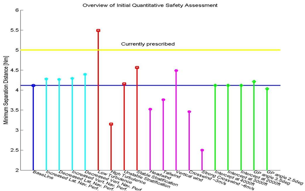
Figure 5.8 Derived Separation Minima under different operational and weather conditions
