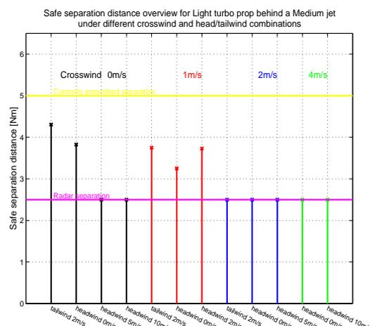
Figure 5.14 Safe separation distance for a Light Turbo Prop behind Medium Jet
