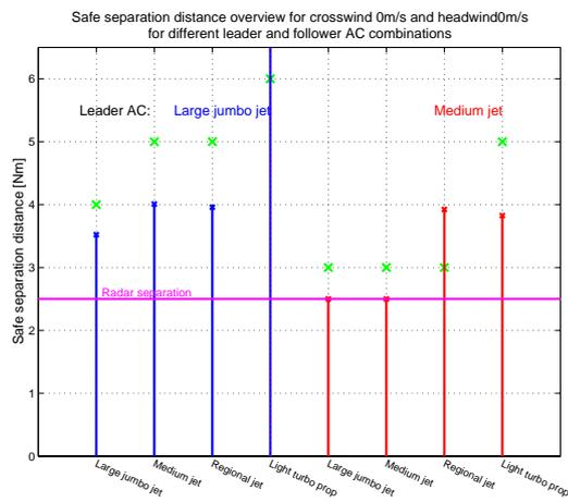
Figure D.2 Safe separation distance for the situation without any wind
