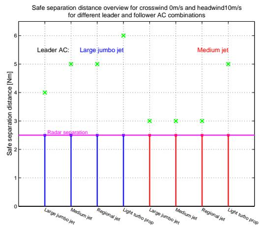
Figure D.4 Safe separation distance for a headwind of 10 m/s and no crosswind
