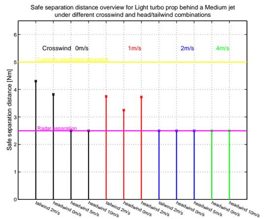
Figure C.4 Safe separation distance for a Light Turbo Prop behind Medium Jet
