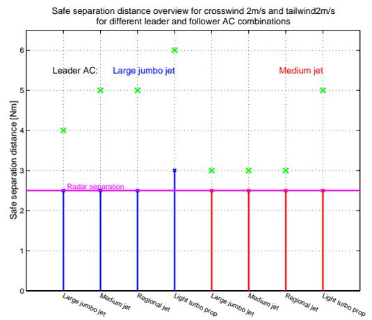
Figure F.4 Safe separation distance for a tailwind of 2 m/s and a crosswind of 2 m/s
