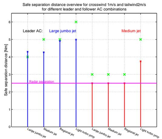
Figure F.3 Safe separation distance for a tailwind of 2 m/s and a crosswind of 1 m/s
