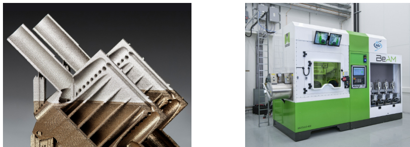
Figure 3. (left) A multi-material additive manufactured part. (right) The DED machine at NLR [12].
