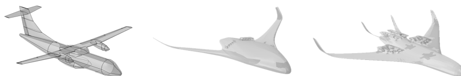
Figure 5. (left) The aerodynamic shape of the ATR-42 conventional aircraft. (middle) A shape similar to the Airbus Zero-e aircraft and (right) a study of a blended-wing aircraft.
