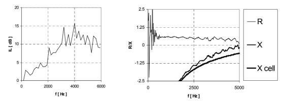
Figure 8a+b Insertion loss (left) and in-situ acoustic impedance, T = 440 °C, M = 0.3, broadband excitation,  $\Delta f = 160$  Hz (a) and  $\Delta f = 20$  Hz (b).
