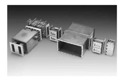
Figure 2 Duct elements of the NLR hot stream liner test facility.
