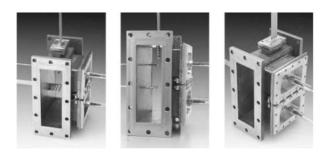
Figure 6 Measurement sections with acoustic (Kulites at right side) and aerodynamic instrumentation for transmission and insertion loss measurements.
