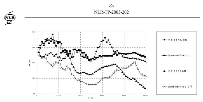
Figure 7 Acoustic signal to flow noise ratio, hard-wall, T = 500 °C, M = 0.35, loud-speakers are switched on or off (flow noise only), broadband excitation,  $\Delta f = 160$  Hz.
