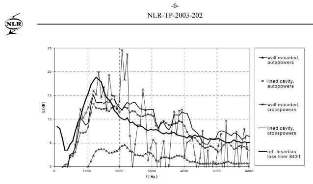
Figure 3 Comparisons of various measured insertion losses in the NLR-FDF, reference liner 8431, flow Mach number is 0.35, broadband excitation,  $\Delta f = 80$  Hz.
