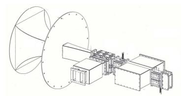
Figure 1 Hot stream liner test set-up with collector/ contraction, source section, measurement section for the incident acoustic field, liner test section with two boxes, measurement section for the transmitted acoustic field and lined exit nozzle.
