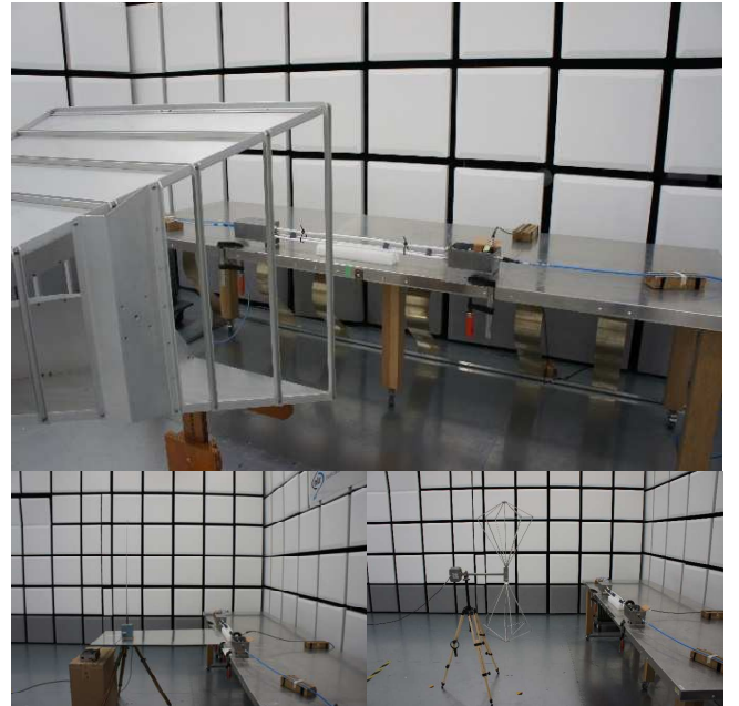
Fig. 5. Pictures of the measurement set-up: a) top picture – with horn antenna, b) lower left picture - with the rod antenna, and c) lower right picture - with the double-ridged horn antenna. In all cases a power feeder is placed 10 cm from the edge of a conducting table, and the antenna 90 cm away from the table.
