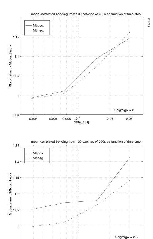
Fig. A.16 A310 mean correlated bending from 100 patches of 250 s as function of time step, for two turbulence intensity levels
