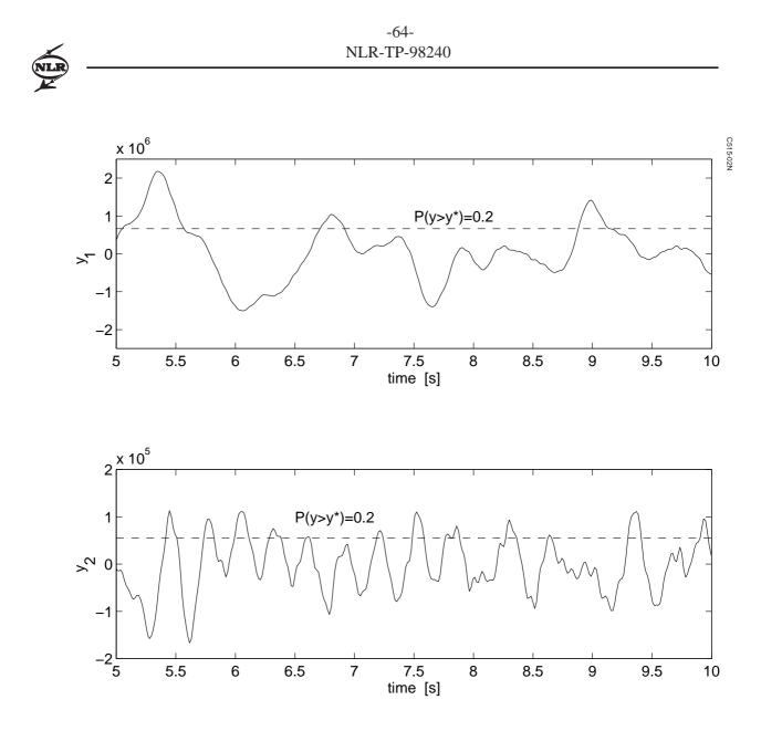
Fig. A.5 Time responses to stochastic gust of two load quantities of an aircraft
