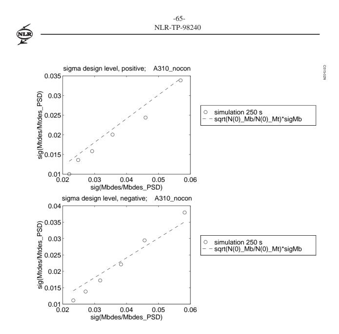
Fig. A.6 A310 torsion design level standard deviation as function of bending design level standard deviation
