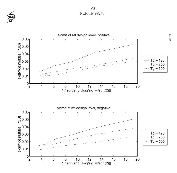
Fig. A.4 Linear A310 torsion moment design level standard deviation as function of turbulence intensity  $\sigma_w$
