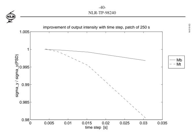
Fig. 6 Improvement of A310 output intensity with time step with respect to theoretical PSD value
