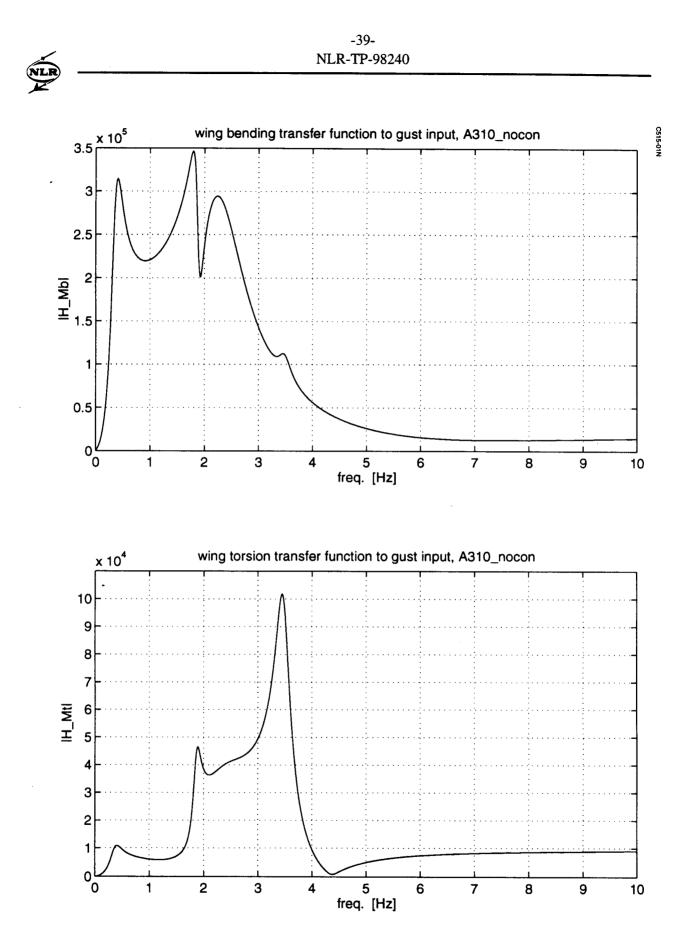
Fig. 5 A310 model transfer functions
