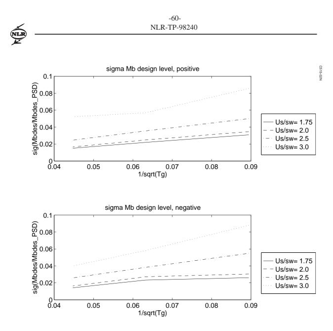
*Fig. A.1* Linear A310 bending moment design level standard deviation as function of turbulence patch length
