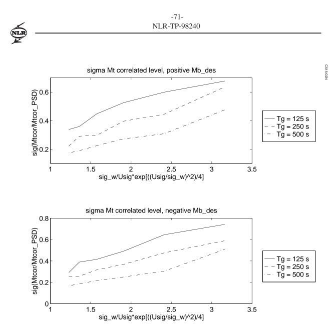
Fig. A.12 Linear A310 torsion moment correlated level standard deviation as function of turbulence intensity  $\sigma_w$
