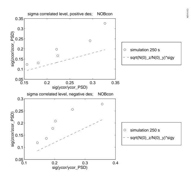
*Fig. A.15* Noback model output *z* correlated level standard deviation as function of output *y* correlated level standard deviation
