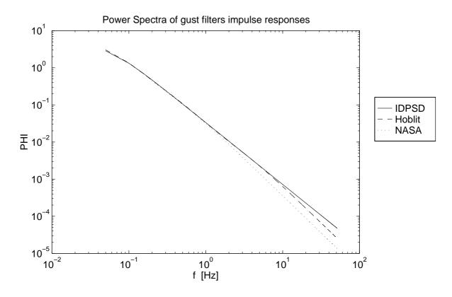
Fig. 7 Power Spectra of three gust filters impulse responses
