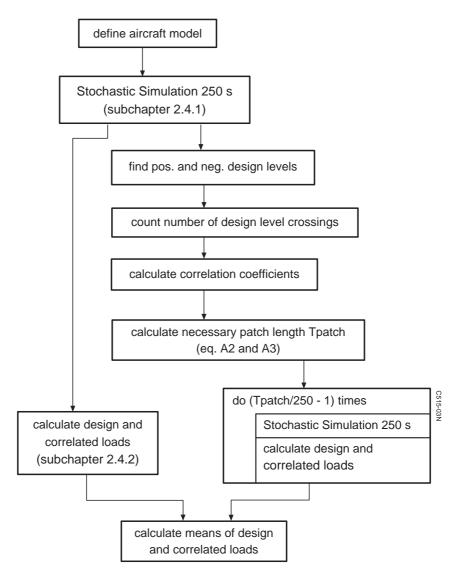
Fig. A.18 The proposed Stochastic Simulation procedure
