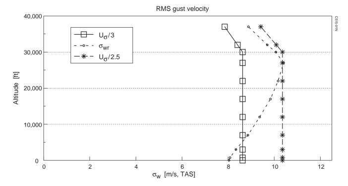
Fig. 2 Three functions of rms gust velocity versus altitude
