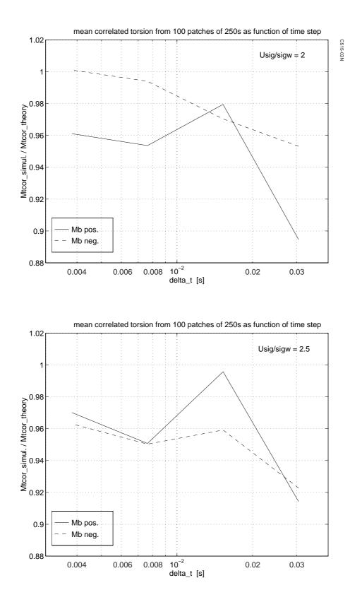
Fig. A.17 A310 mean correlated torsion from 100 patches of 250 s as function of time step, for two turbulence intensity levels
