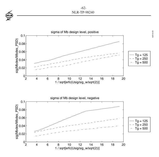
Fig. A.3 Linear A310 bending moment design level standard deviation as function of turbulence intensity  $\sigma_w$
