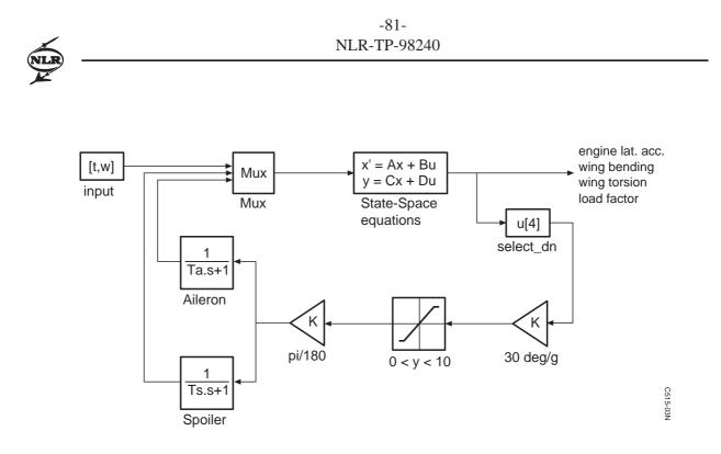
Fig. B.3 A310 model with load alleviation system (from Ref. 6)
