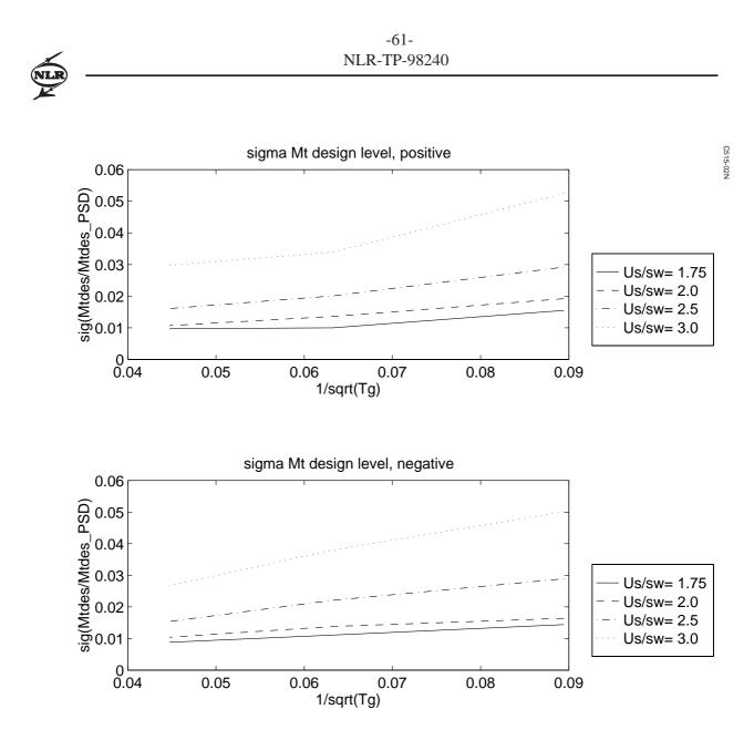
*Fig. A.2* Linear A310 torsion moment design level standard deviation as function of turbulence patch length
