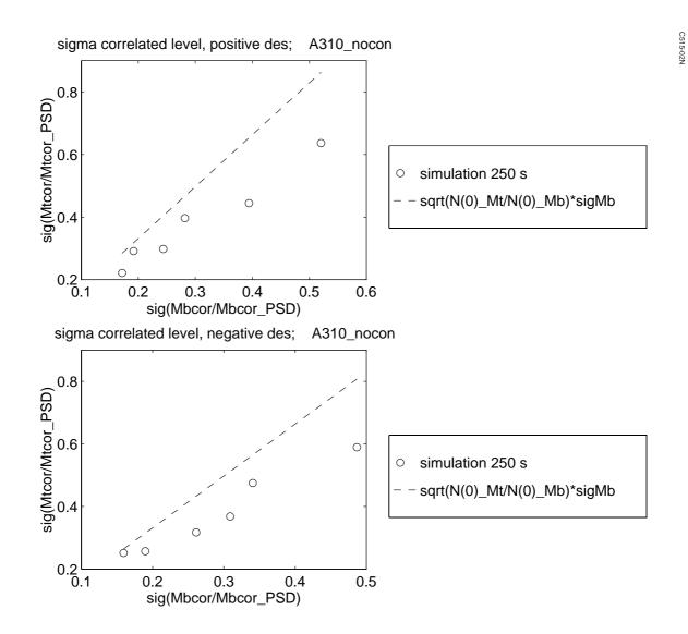
Fig. A.13 A310 torsion correlated level standard deviation as function of bending correlated level standard deviation
