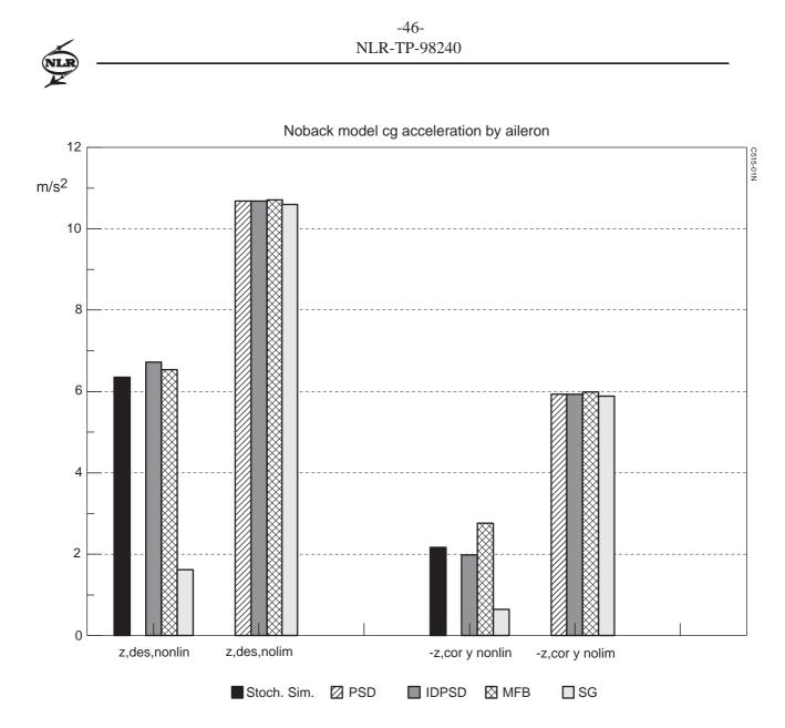
Fig. 13 Stochastic, Deterministic and "standard" PSD results for Noback models
