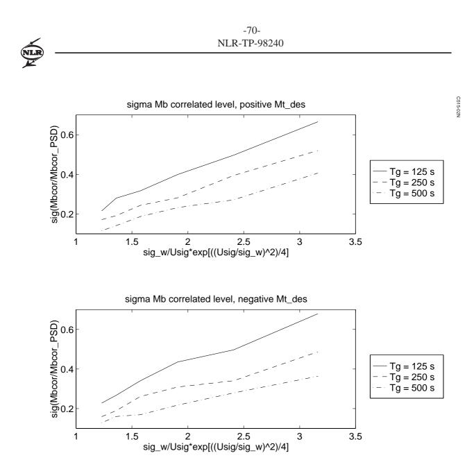
Fig. A.11 Linear A310 bending moment correlated level standard deviation as function of turbulence intensity  $\sigma_w$
