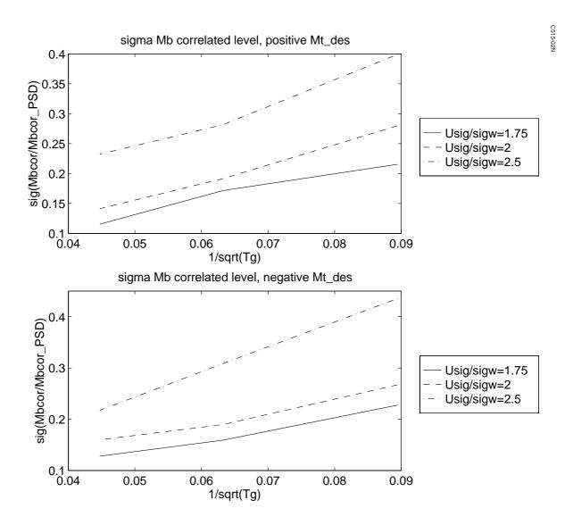
*Fig. A.9 Linear A310 bending moment correlated level standard deviation as function of turbulence patch length*
