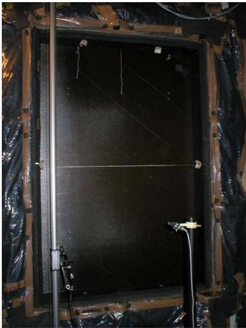
Fig. 9. Dassault set-up for TL measurement of the FUBACOMP panel
