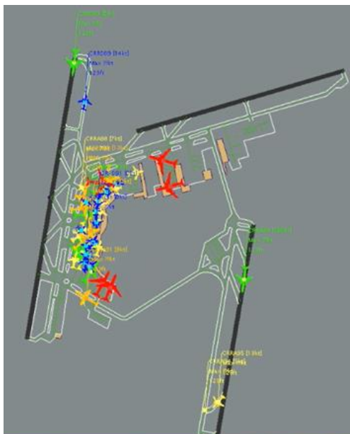
Figure 2. Simulation with AirTop: Aircraft ground movements [Source: Royal NLR].
