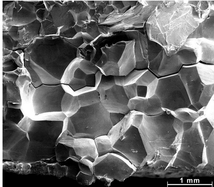
Figure 5 FEG-SEM fractograph at, and near, the external surface of a sample from the sawn-off slice. The fracture is almost entirely intergranular
