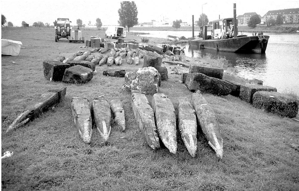
Figure 1 Some of the piles, pile-shoes and stone blocks recovered from the Maas riverbed: photograph courtesy of R. Kroes
