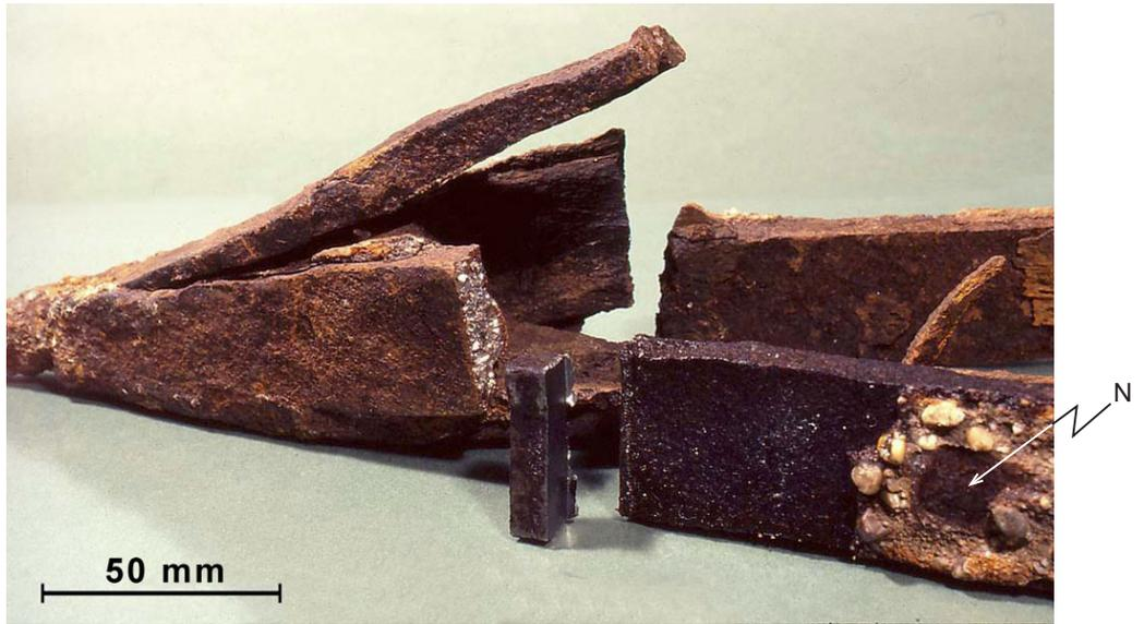
Figure 3 The broken pile-shoe with a sawn-off slice containing the upper fracture surface of the recent break. "N" indicates the head of a nail driven through a hole in the bar in order to attach it to the wooden pile
