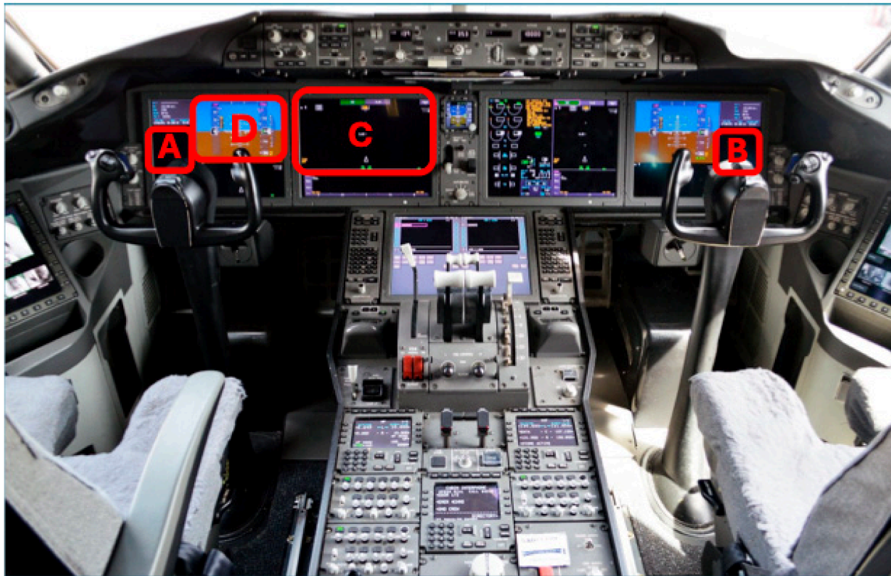
Figure 3. Highlighted B787 cockpit display elements for the 5 use cases. Highlighted Areas: A and B = Text area (e.g., for CPDLC (Controller-Pilot Data-Linked Communication)), C = Multifunction Display (MFD), D = Primary Flight Display. Human–AI Interaction Areas by Use Case: UC1: Voice to Text = A + B; UC2: RWY and Taxiway = A + B, C for TWY map; UC3: Major Re-Routing = A, B, C for route map and XAI; UC4: Safety Advisor = A, B, C; UC5: Startle Response Support = C + D.
