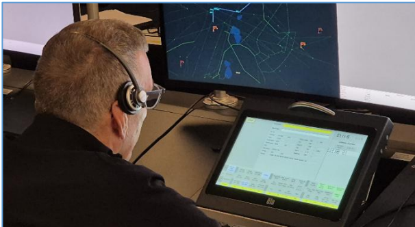
Fig. 8: Pseudo-pilot Working Position with CPDLC Display
