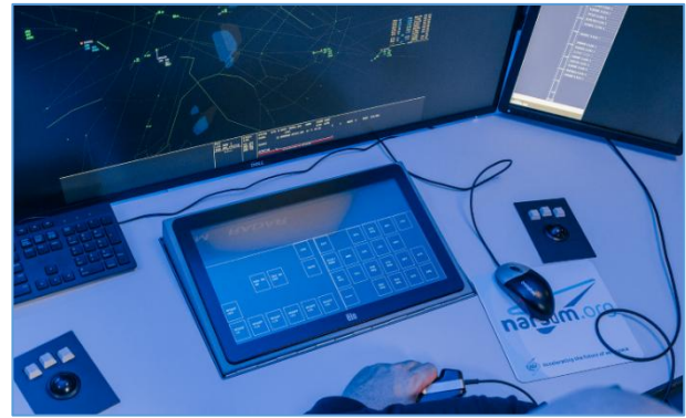
Fig. 5: Input Devices on the CWP (NARSIM).
