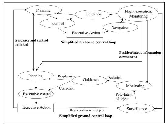
Figure 3 - Exchange of information between airborne and ground guidance and control processes.
