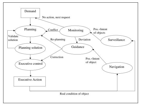
Figure 2 - A generic model of a guidance and control loop in an ATM process
