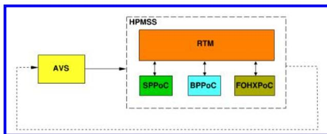
**Figure 13. Decoupling of flight mechanical part of the simulator from internal heat and power management system components; feedback of system/component status and outputs is foreseen for the future.**
