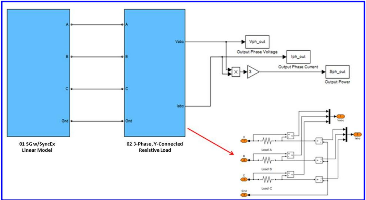
Figure 3. 2-Stack synchronous generator model (top level).
