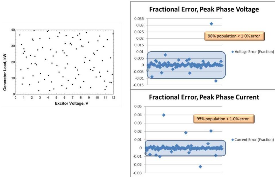
**Figure 7. Corroboration of surrogate polynomial model to the generic generator physics-based model showing the random inputs and fractional error for outputs, peak phase voltage and current.**
