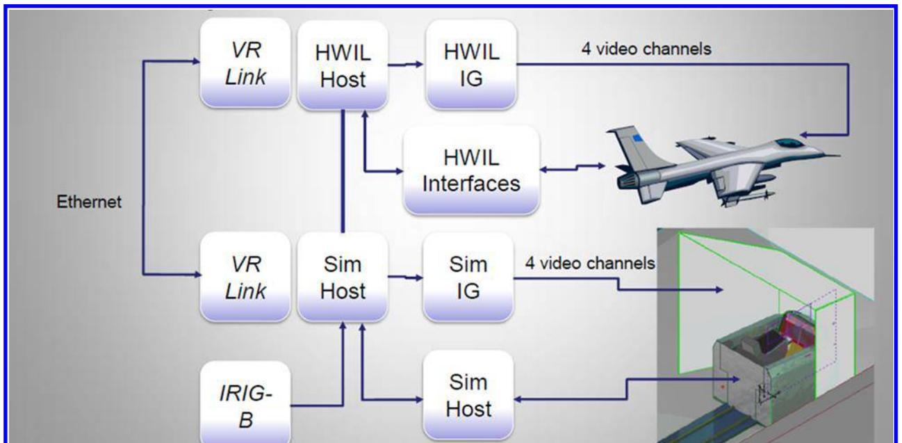
Figure 18. Integration of the airframes and the flight simulation computational hardware developed by Protobox, LLC.
