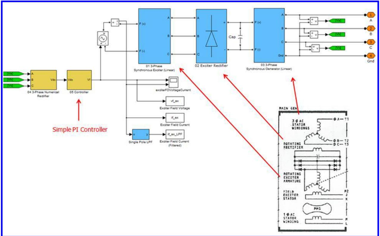
Figure 4. 2-stack synchronous generator model (subsystem level).
