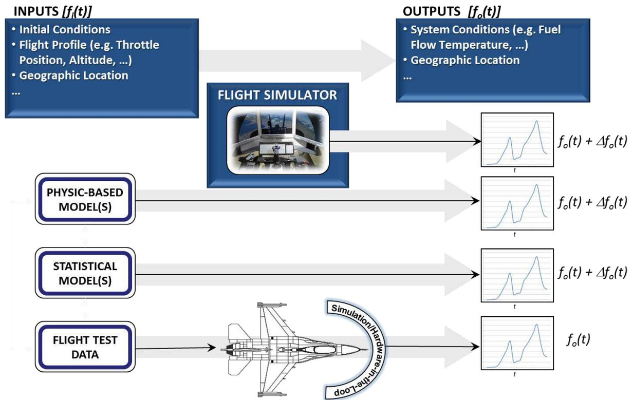
Figure 19. IEPM Laboratory validation testing approach.
