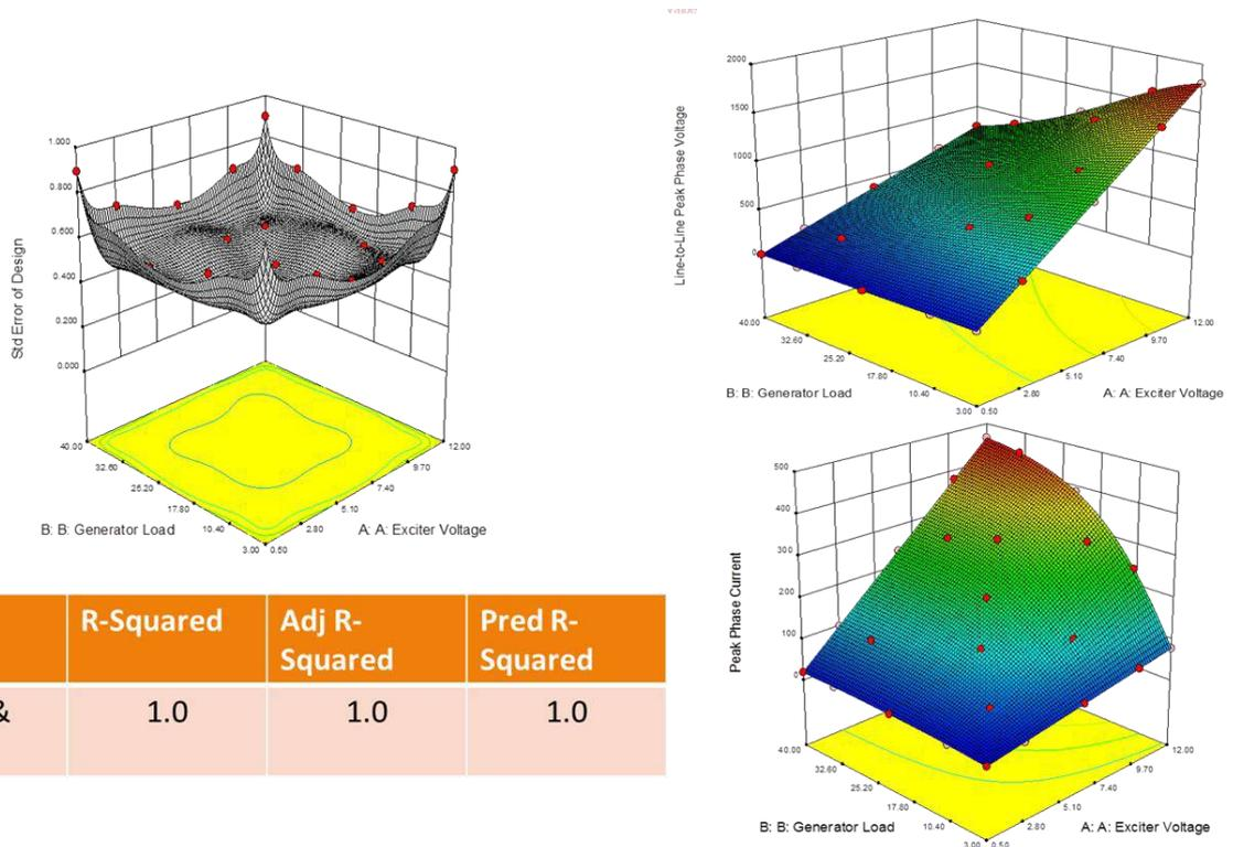
**Figure 6. Quartic statistical model standard error and resulting voltage and current response surfaces derived from generic generator model.**
