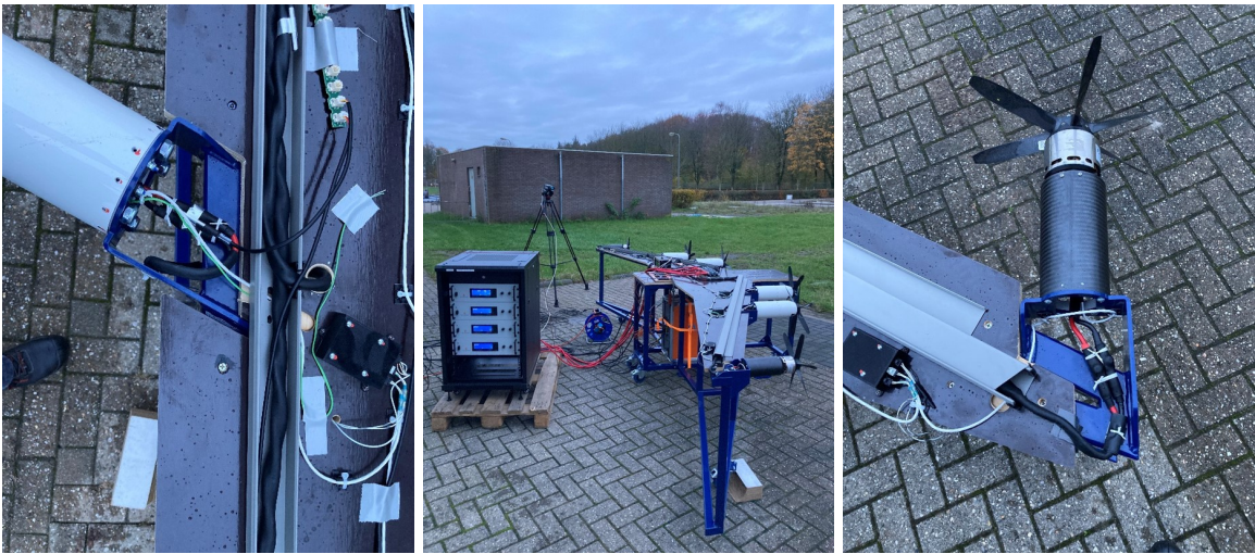
Figure 14. The iron-bird of the DEP-SFD2.
