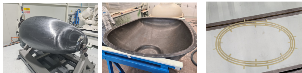
Figure 3. Manufacturing result of inner tank (left), top outer tank half (middle) and circumferential tank spacer (right).
