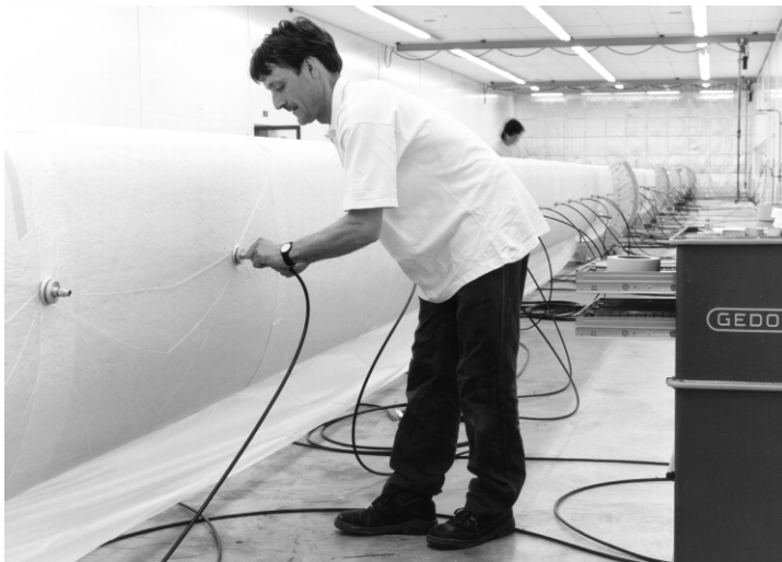
Fig. 5 Preparation of vacuum bag prior to curing
