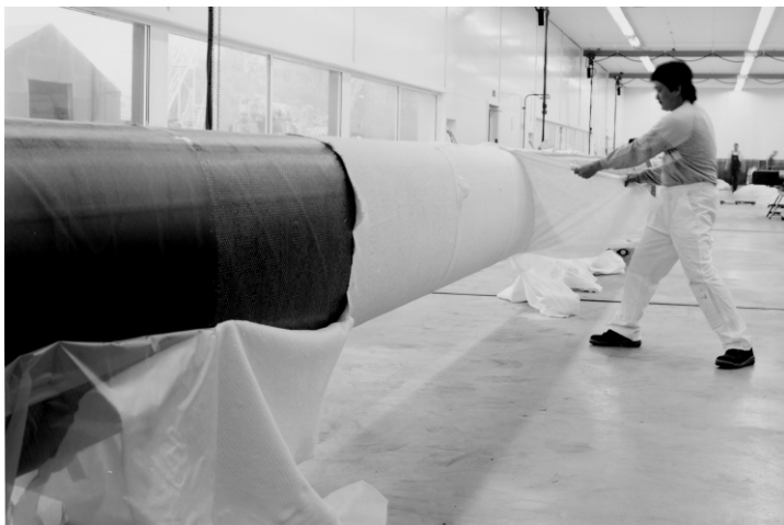
Fig. 6 Removal of vacuum bag and bleeder material after curing
