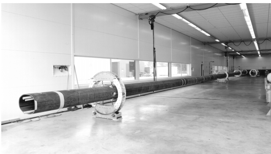
Fig. 4 Mast on rotation supports during laminating
