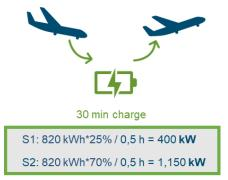
Figure 17 - Overview of charging requirements for scenario 1 and 2
