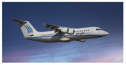
Figure 9 - BAe146 retrofit Wright Electric all-electric aircraft (source: Wright Electric)
