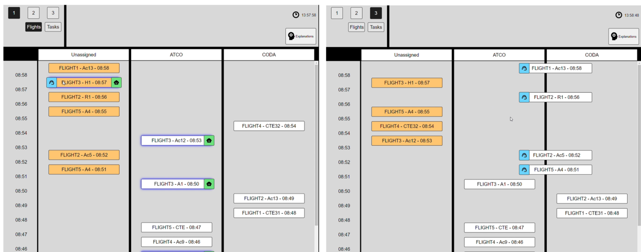
Fig. 5 Examples of higher-fidelity research-prototype screens derived from the mock-ups and used for interactive prototype review and iteration with the expert ATCOs during workshops. Left: In the manual mode, only the ATCO is the allocation agent and the ATCO can assign or leave unassigned the relevant flights and tasks. Right: In the auto-
