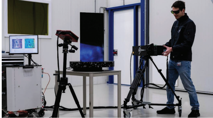
Figure 9: The automatic inspection system for curved composites with from left to right: the laser ultrasonic pc, the 3D scanner, the rotation table with a curved component, the laser ultrasonic scanner and the first author.
