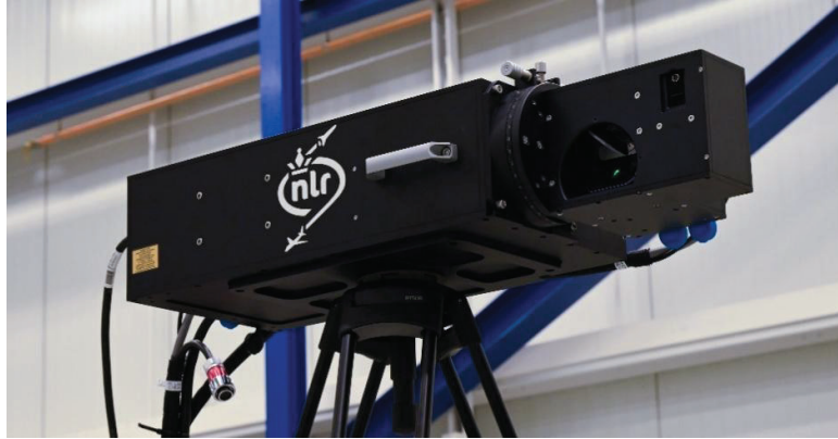
Figure 1: The angular laser ultrasonic system. On the right side a green aiming laser is visible on the steering mirror.
