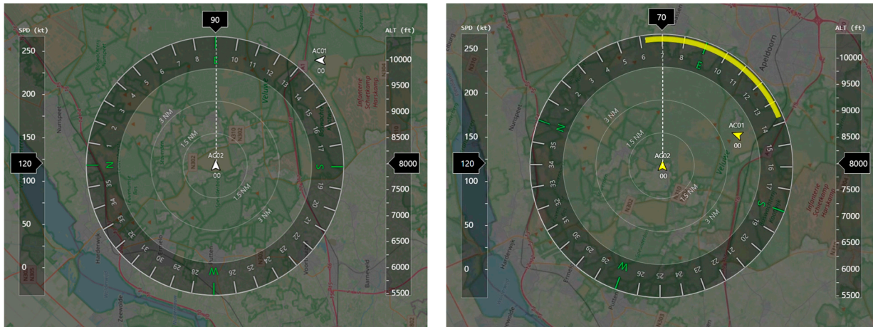
Figure 1. RWC avoidance bands guidance display (track-up): without active bands (left figure) and with active bands (right figure).
