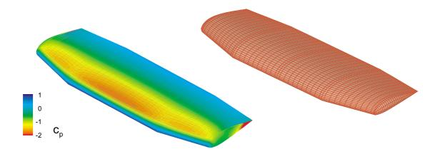
Fig. 4 Computational grid and pressure distribution without boundary layer effects on clean wing at cruise condition (  $h = 12 \text{ m}, \alpha = 5^{\circ}, \delta_F = 0$ )
