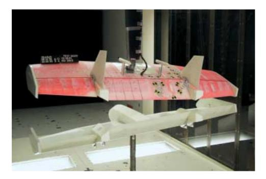
Fig. 6 Seabus wind tunnel model with additional instrumentation
