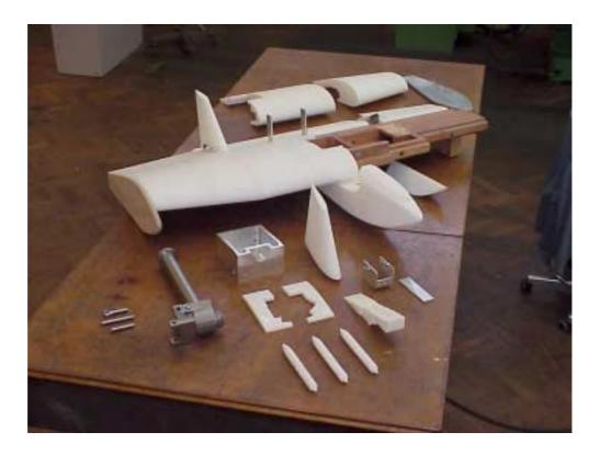
Fig. 8 Seabus wind tunnel model components before assembly
