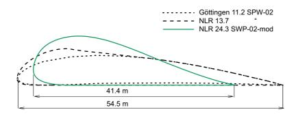
Fig. 2 SPW-02 and SPW-02-mod airfoils designed by NLR
