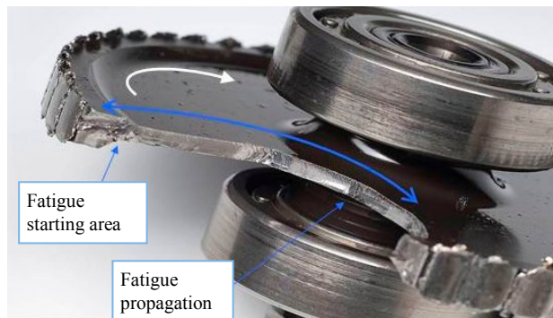
Fig.7 Gear 1 fracture surface; the blue arrow marks the area with fatigue indications and the white arrow indicates the direction of rotation (note missing teeth)
