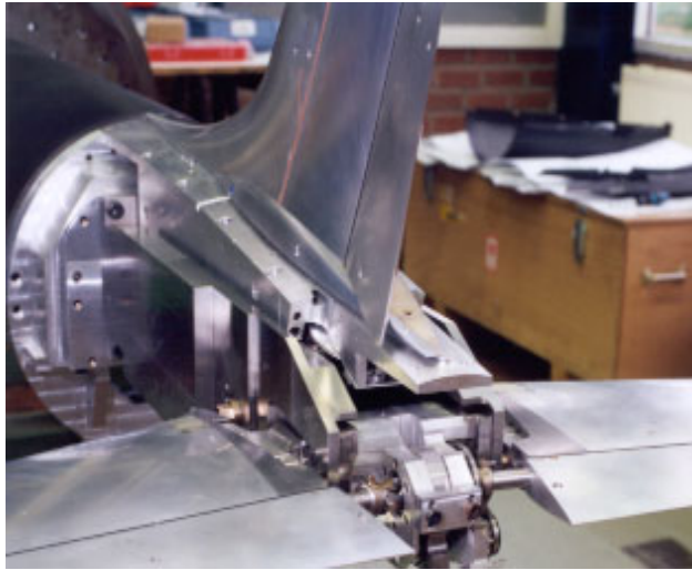
Fig. 3 Rear fuselage of model with remotely controlled elevators and rudder (NLR)
