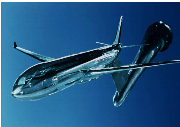
Fig. 4 Cryogenic model with remotely controlled horizontal tail plane (ONERA)
