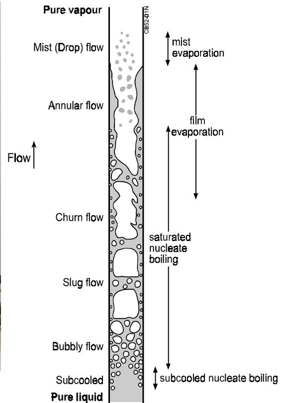
FIGURE 4. Flow Patterns and Boiling Mechanisms for Up-Flow in a Vertical Line on Earth
