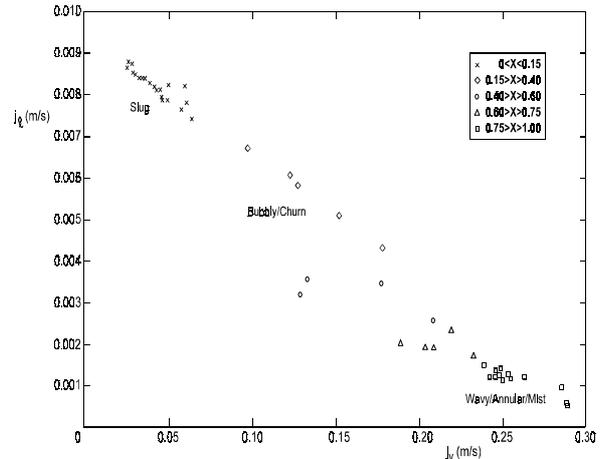
FIGURE 18 Flow Patterns Derived from TPX I Vapour Quality Sensor Data
