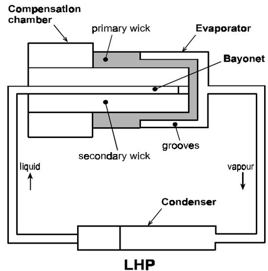
FIGURE. 2 Schematics of Loop Heat Pipe
