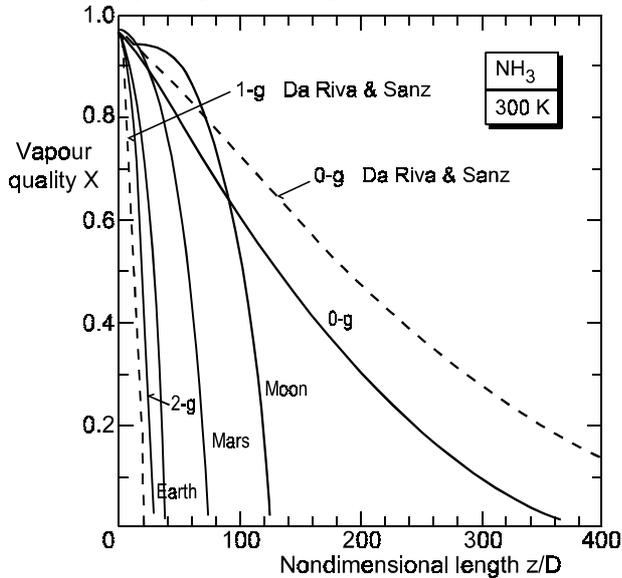
FIGURE 13. Vapour Quality Along the 16.1 mm Duct for Ammonia at 300 K, 1 kW, for All Gravity levels
