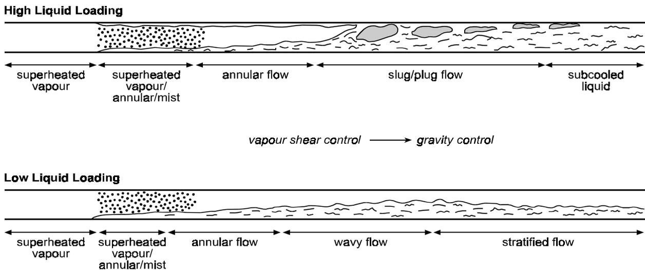
FIGURE 6. Horizontal Condenser Line on Earth
