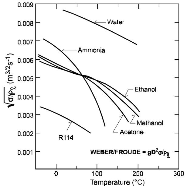
FIGURE 7.  $(\sigma/\rho_l)^{1/2} = D \cdot g^{1/2} / (We/Fr)^{1/2}$  Versus Temperature
