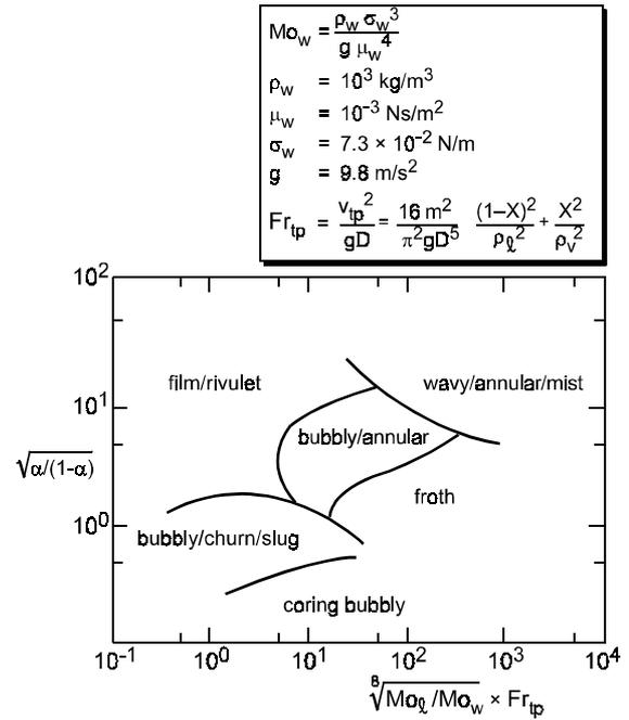
FIGURE 8. Flow Pattern Map for Vertical Down Flow
