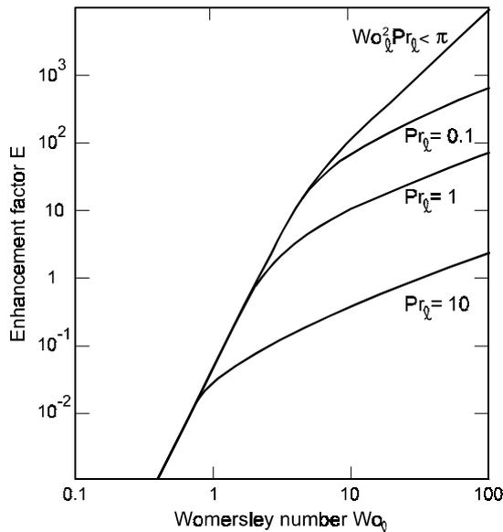
FIGURE 3. Enhancement Factor E Versus Wo and Pr
