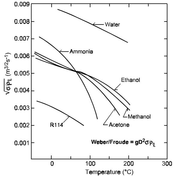
FIGURE 2.  $(\sigma/\rho_l)^{1/2} = D \cdot g^{1/2} / (We/Fr)^{1/2}$  Versus Temperature
