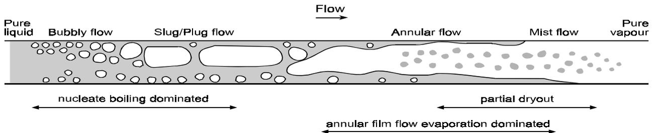
FIGURE 5. Horizontal Evaporator Line on Earth
