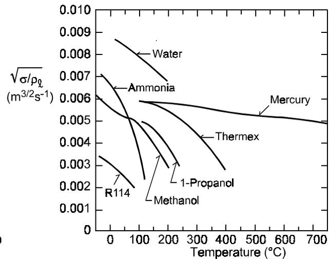
FIGURE 10.  $(\sigma / \rho_l)^{1/2} = Dg^{1/2} / (We / Fr)^{1/2}$  Versus Temperature
