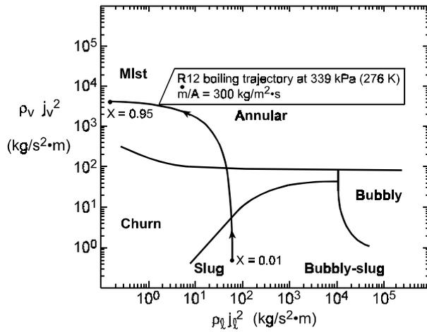
FIGURE 7. Flow pattern map for vertical flow
