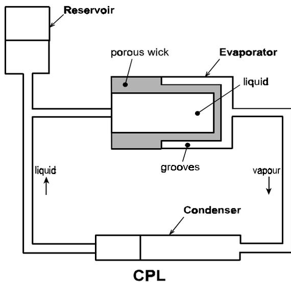
FIGURE. 1 Schematics of Capillary Pumped Loop
