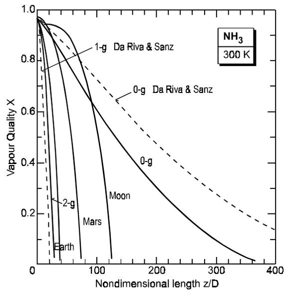
**FIGURE 4.** Vapour Quality Along the Reference Duct
