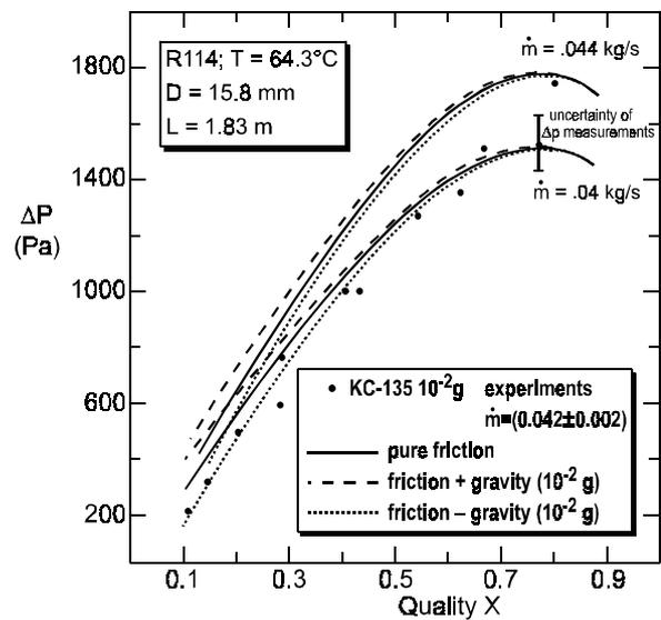
FIGURE 12. Measured and Predicted Adiabatic Pressure Drops
