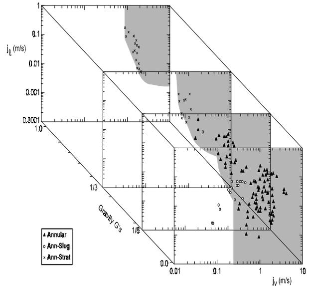
FIGURE 14. Annular Flow: Gravity Dependent Three-Dimensional Flow Pattern Map
