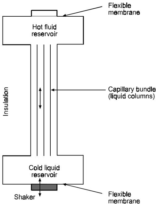
FIGURE 1. Synchronised Forced Oscillatory flow HTD
