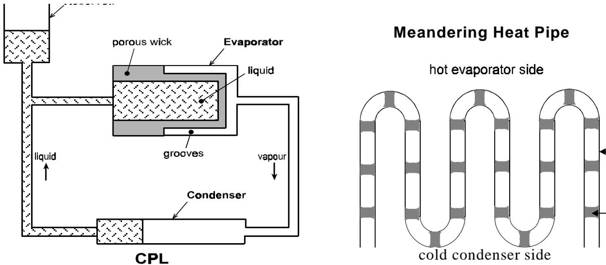
FIGURE 5. Schematics of a Capillary Pumped Loop (left) and a Meandering Heat Pipe (right)
